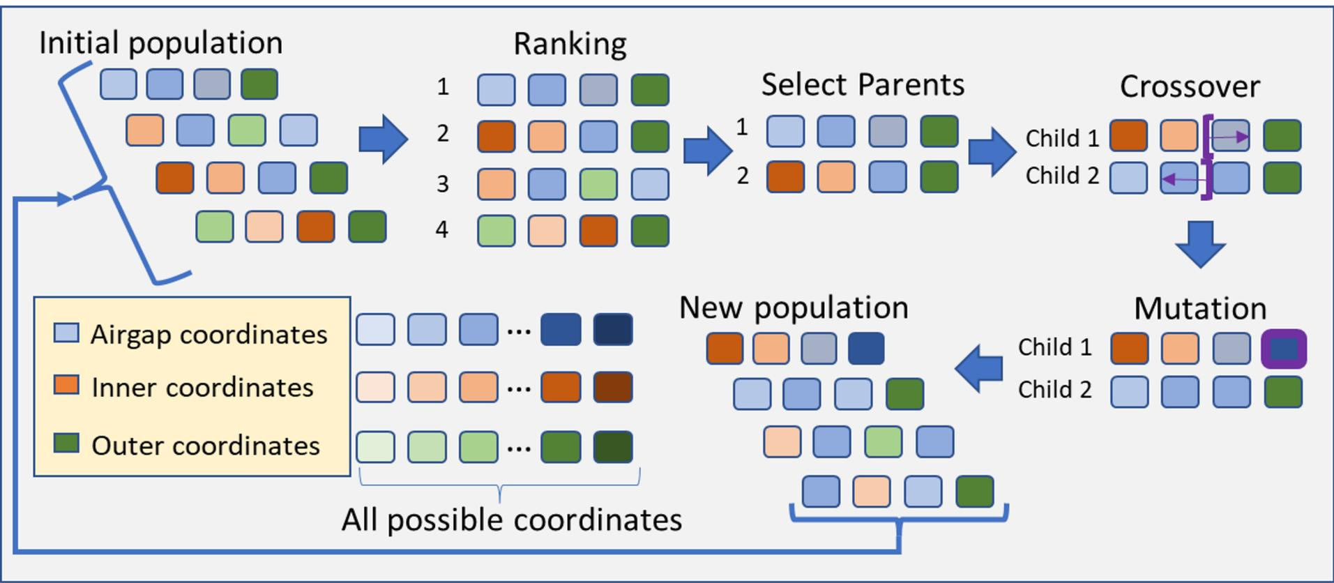
Genetic algorithm for selecting the best sensor placements for detecting inter-turn winding fault
