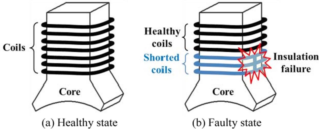
Occurs when insulation on the coil fails causing a short.
