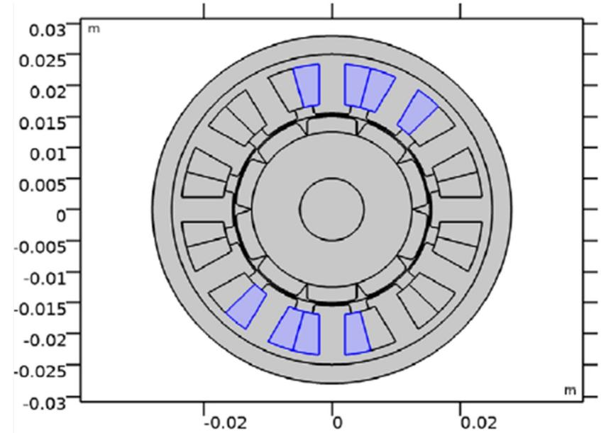
Insert fault by changing the coupling equivalent circuit of motor.
