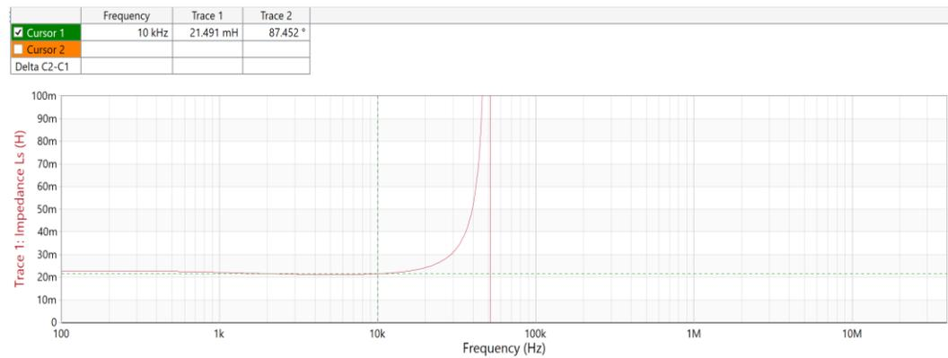
Fig. 30. Inductance vs frequency plot of LTCC based transformer. [Image by author]
