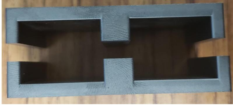
Fig. 11. Planar transformer core- perspective. [Image by author]
