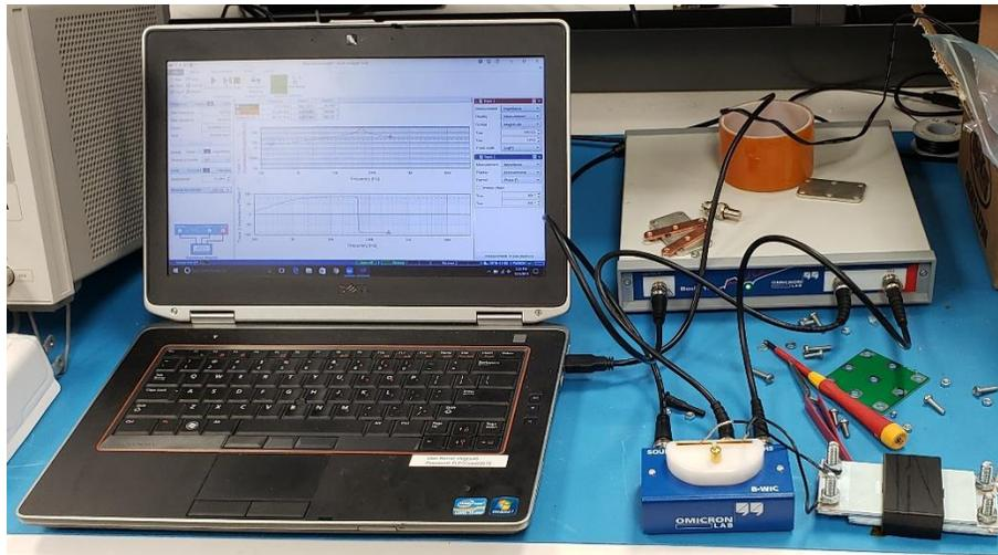
Fig. 28. Impedance analysis test setup. [Image by author]
