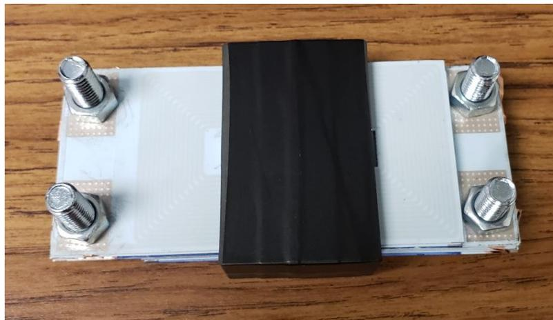
Fig. 25 Assembly of LTCC transformer. [Image by author]
