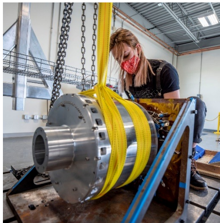
(left) 15,000 rpm, 1-MW slotless PM motor, (center) 300KW machine assembled and (right) tested on PRDC testbed
