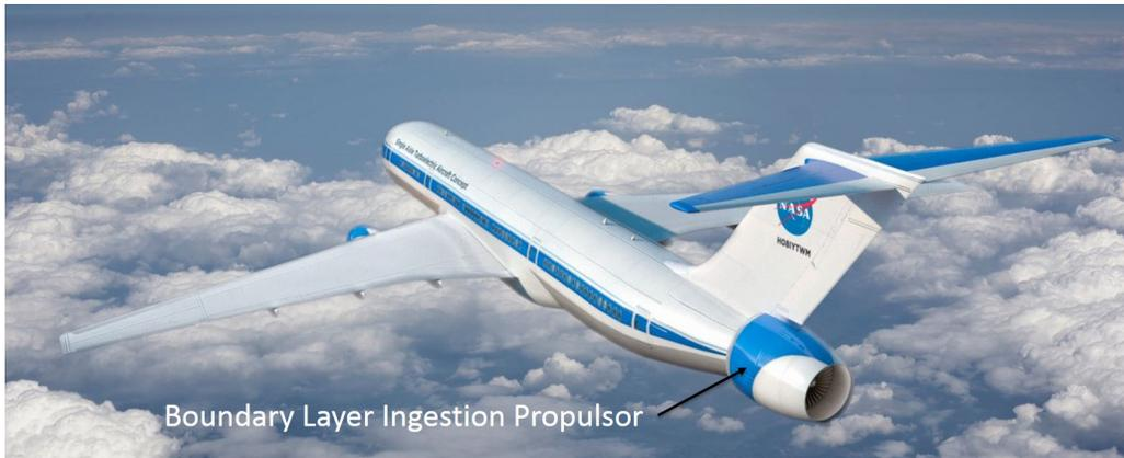
Figure 5.8: STARC-ABL concept. (NASA photo).
