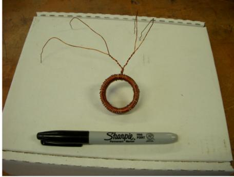
(a) Vacoflux48 core with  $N=65$  bifilar windings.
