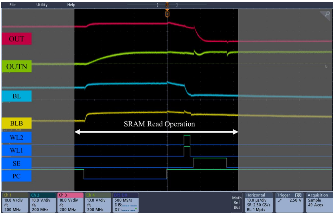
Fig. 56. Reading logic '1' at VDD=10 V and Temperature=400°C.
