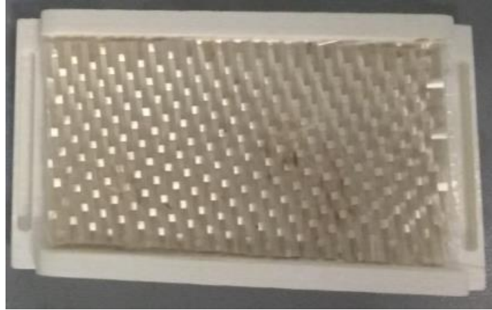
Fig. 46. Image of the Nextel fiber-glass fabric on the base of the CMC housing structure.
