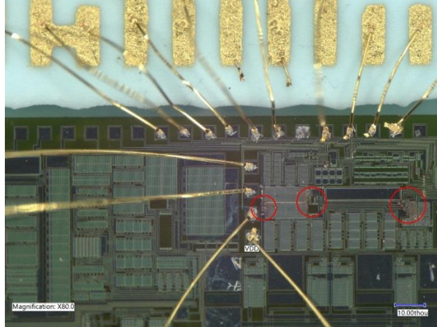
Fig. 84. Visible damage (red-circled) on the reference circuit die due to VDD trace blowing up during 350°C testing with a static current draw of 35 mA at VDD = 30 V.
