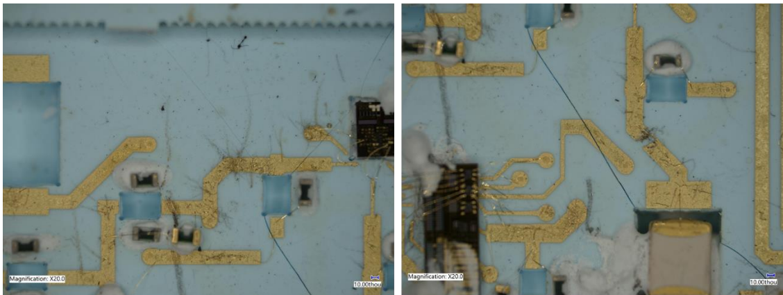
Fig. 71. Visible cracks on the RUK module post-spin-testing.
