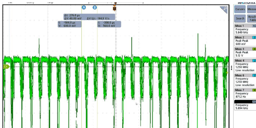
Fig. 69. Observed distortion of the demodulated output for 200 mV applied input to the RUK SiC op amp.
