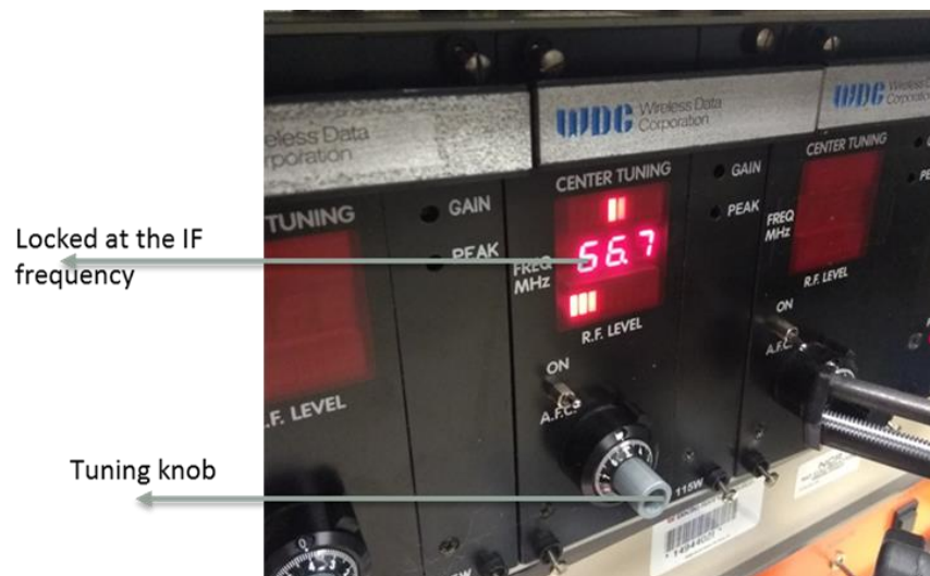
Fig. 67. Front-side view of the receiver unit locked at the intermediate frequency (IF). The output from the telemetry receiver can be observed on the oscilloscope. The signal frequency from the telemetry receiver output should match the frequency of the WB oscillator. To verify the receiver system functionality, a low DC voltage of 100 mV has been applied to the signal conditioning op amp input at a supply voltage of 12 V. The low DC voltage resembles the output
