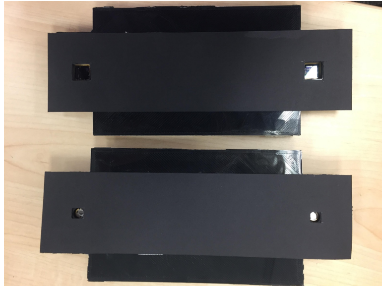
Figure 5.16: Image of 3D-printed holders that kept the AlGaIn/GaN (top) and commercial (bottom) photodetectors in place on the fuel grain.
