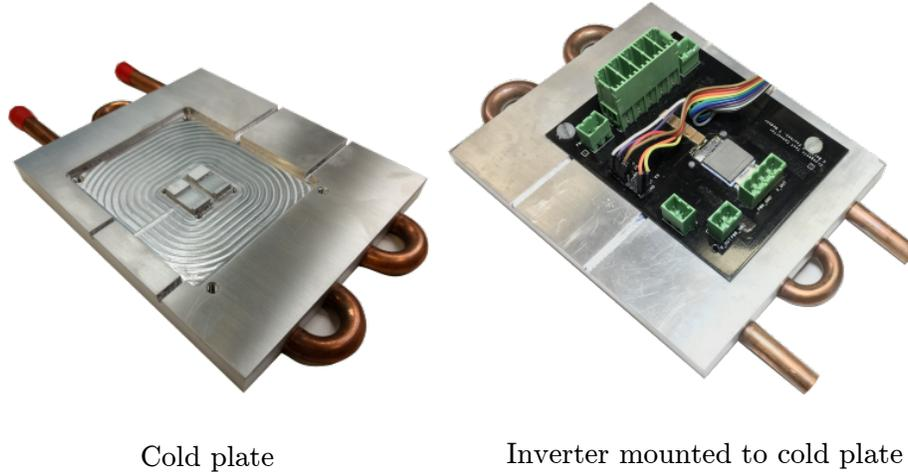
Figure 4.8: Milled cold plate and cold plate with the FCML inverter.
