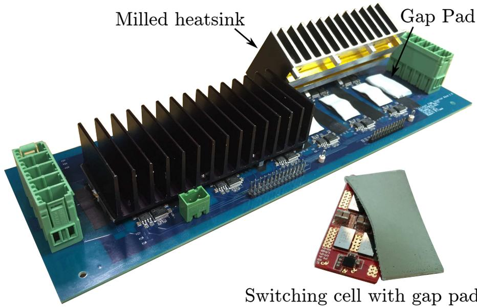
Figure 3.11: 13-level inverter with heatsink.
