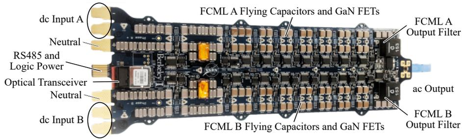
Figure 5.30: Generation 3 ILM. Dc link capacitance is moved to the backplane providing room for POF transceiver [150].
