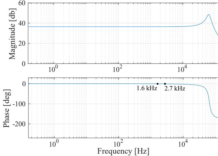
Figure 5.22: Amplitude and frequency response for buck converter/FCML with  $10 \mu\text{H}$ ,  $0.6 \mu\text{F}$  filter stage.
