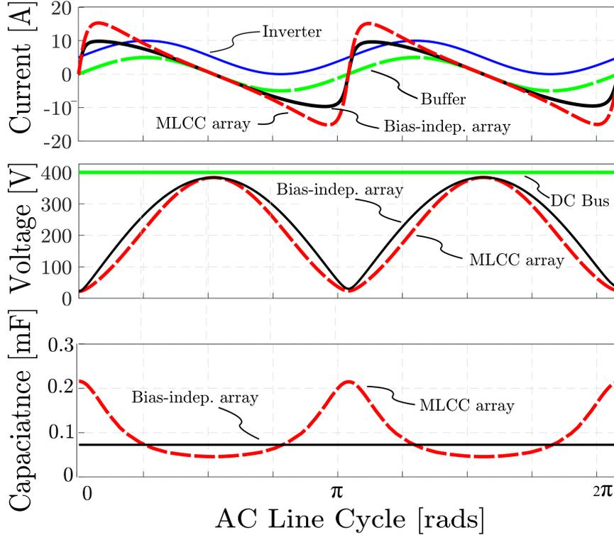
Figure 2.16: Operating waveforms for capacitor array, buffer and inverter. The peak currents of the MLCC array are significantly higher than the peak currents for an ideal capacitor array due to the large change in capacitance of the MLCC array over the line cycle.
