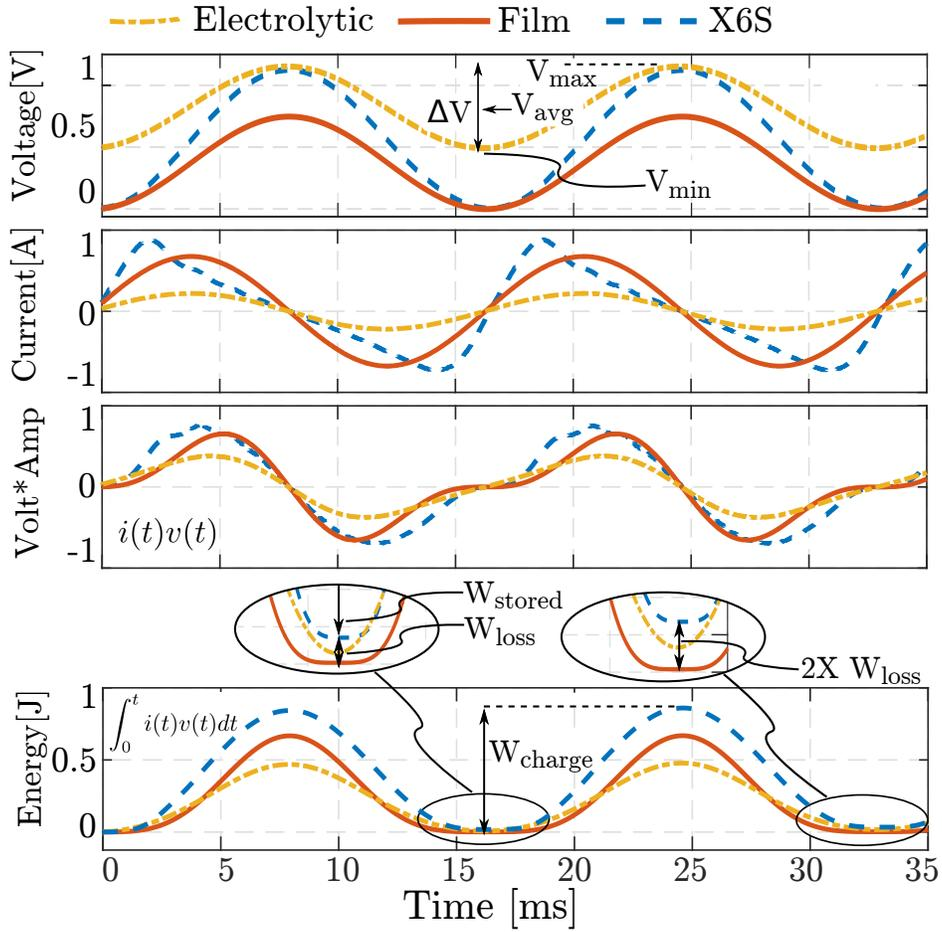
Figure 2.6: Experimental test waveforms for electrolytic, X6S ceramic and metallized polyester capacitors.
