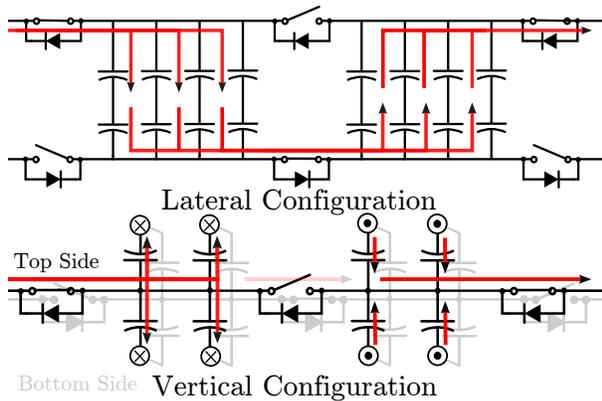
Figure 5.26: Comparison of the current path for lateral and vertical switching cell configuration.
