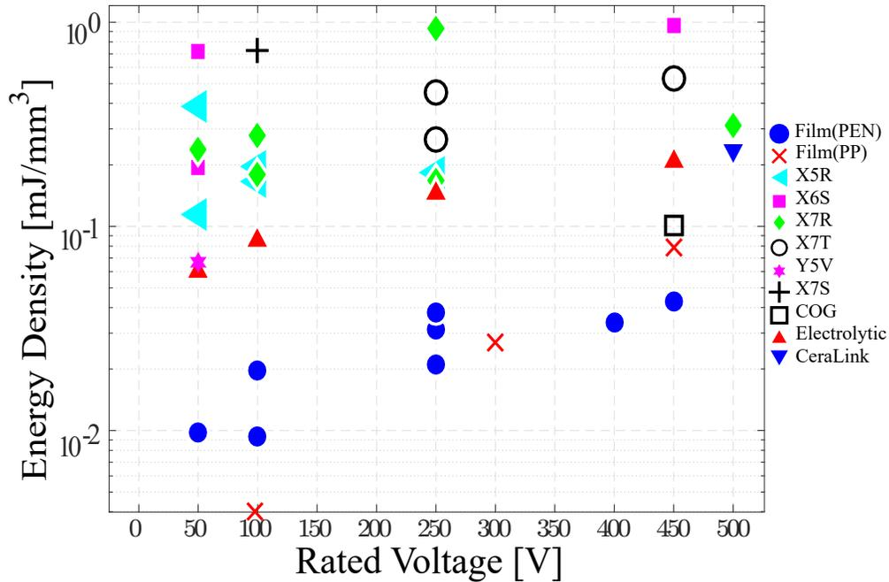
Figure 2.7: Measured capacitor energy density with film capacitors ranking among the lowest energy density and ceramics ranking among the highest.
