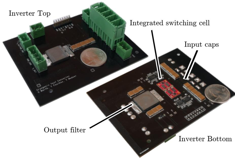
Figure 4.7: Top and bottom view of 3-level inverter.
