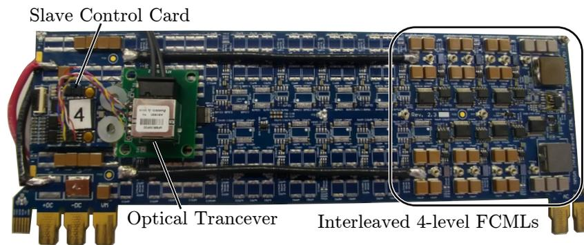
Figure 5.35: Gen 3, 10-level ILM bypassed to four levels for drive development. Optical transceiver added to slave control card.
