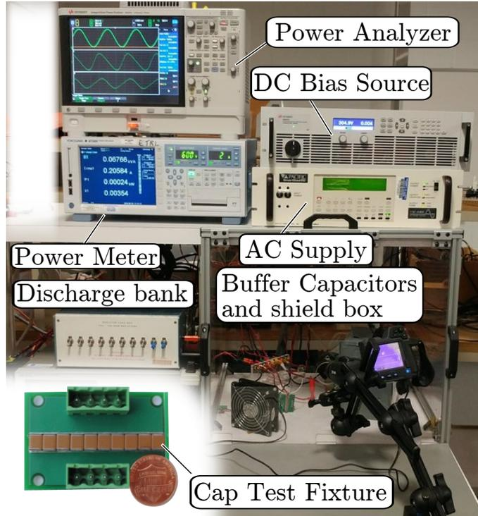
Figure 2.5: Experimental test setup and capacitor test fixture with 10 MLCCs.
