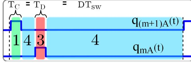
(b) For  $D < \frac{1}{N-1}$  the charge and discharge is proportional to  $D$ .
