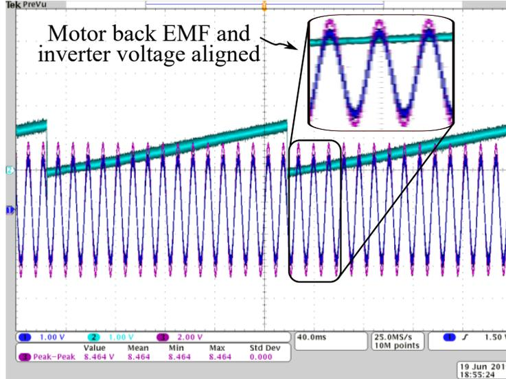
Figure 5.14: Validation of alignment between drive position reading and motor magnetic position.
