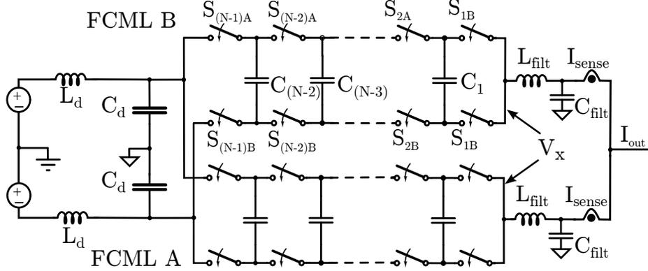
Figure 5.3: Schematic of power path for interleaved inverter module. Current sensing and PWM generation for each module are handled by slave FPGA controller located directly on the module.
