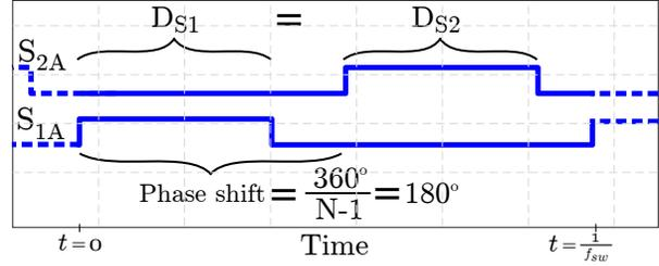
Figure 4.2: High-side gate signals for 3-level FCML driven with PSPWM.
