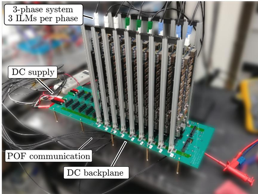
Figure 5.38: Third-generation inverter system assembly with 3 inverters per phase for a total of 9 inverters.
