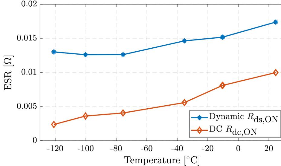
Figure 4.3: Measured dc and dynamic  $R_{ds,ON}$  of EPC2034 over temperature. While dc measurements suggest a  $\approx 76\%$  reduction, the dynamic on-state resistance only decreases by  $\approx 27\%$ , and shows a slight increase below  $-80\text{ }^{\circ}\text{C}$  [13, 103].
