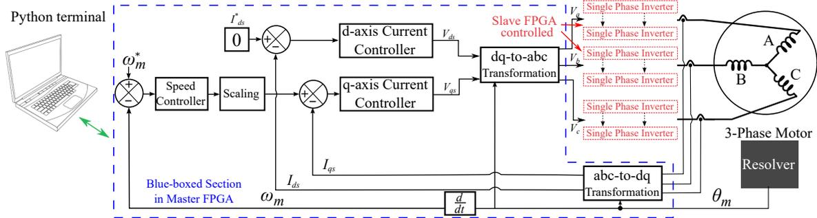
Figure 5.19: Control structure for FCML-based motor drive. Drive-level control is accomplished in the master controller while PWM generation and current balancing is handled in the slave controller.
