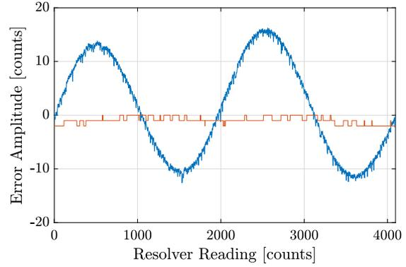
Figure 5.18: Error in position measurement before and after implementation the tuning circuit in Fig. 5.17.
