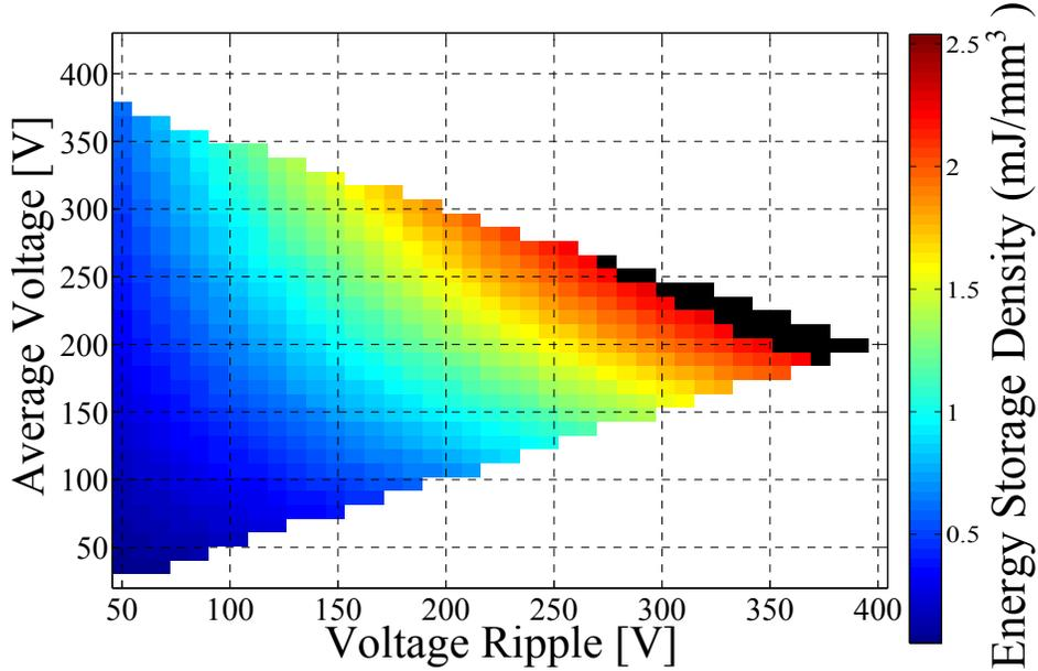
Figure 2.11: Energy buffering density for a bias-independent  $2.2 \mu\text{F}$  capacitor with the same dimensions as #23. Black region indicates top 10% of energy density. It can be observed that, under the constraint of the capacitor and switch voltage ratings, the maximum energy density is obtained by maximizing the voltage ripple and maintaining the highest possible voltage.
