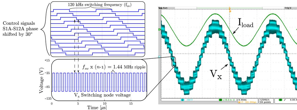
Figure 3.15: Simulation of phase-shifted switch PWM, switching node ripple frequency, and experimentally measured switching node voltage.
