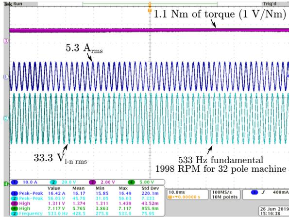
Figure 5.49: Line current and voltage when driving the 32 pole ThinGap motor at 2 kRPM. This equates to 15,990 RPM for a 4-pole machine
