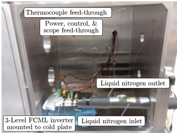
Figure 4.9: Vacuum chamber with converter configured for testing. Thermocouples, power and LN2 were passed through feedthroughs to the converter.
