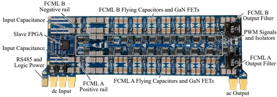
Figure 5.29: Generation 2 ILM. Dual, interleaved 10-level FCML design reduces impact of dynamic  $R_{dsON}$ . Separating signal and power traces forces opposite polarity dc supply rails on FCML A and B.
