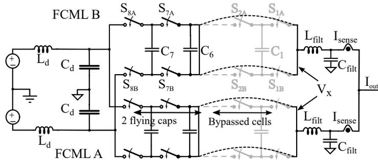
Figure 5.31: Schematic for 9-level interleaved module (ILM) module bypassed to 3 levels for drive development.
