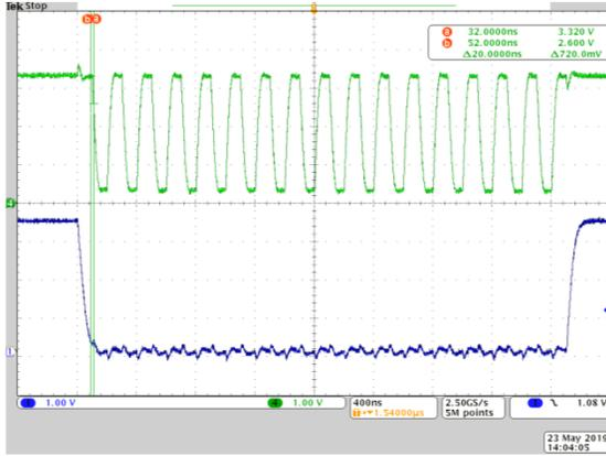
Figure 5.24: Filtered clock and chip-select single-ended signals and the input of the current sense ADC on the 10-level ILM.
