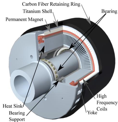
Figure 5.1: 1 MW permanent magnet, outer rotor motor developed at UIUC [128].
