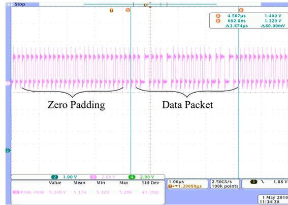
Figure 5.25: Manchester asynchronous serial with zero padding transmitted via optical link.
