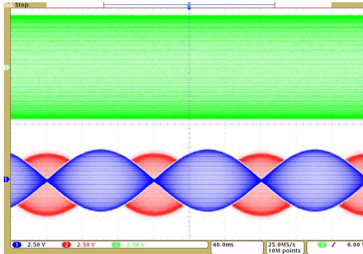
Figure 5.11: Resolver excitation signal (top), sine and cosine feedback signals as motor shaft rotates (bottom).
