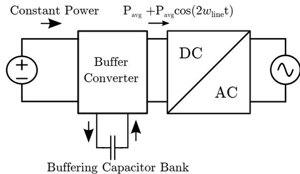
Figure 2.2: Energy buffering circuit of single-phase inverter.
