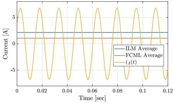
Figure 5.43: Motor phase current as well as ILM and FCML average values read from master controller over SPI.
