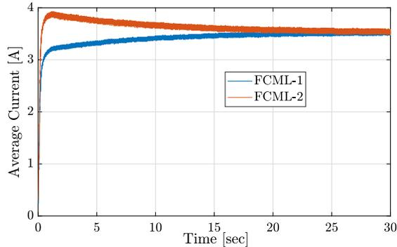
Figure 5.8: Measured 160 millisecond running average of rectified current measurement from FCML-1 and FCML-2.
