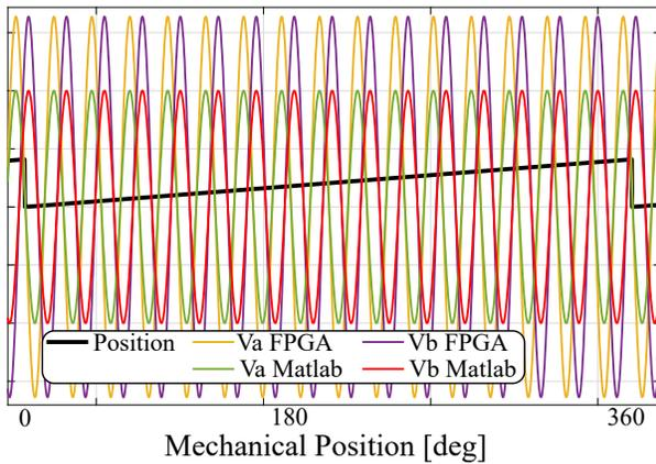
Figure 5.12: Numerical comparison of FPGA and MATLAB calculated  $dq$  to  $ABC$  transformation.
