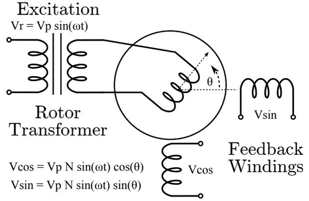
Figure 5.10: Functional schematic of brushless classical resolver.
