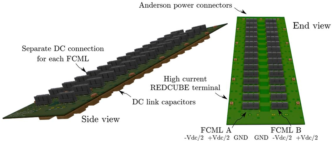
Figure 5.37: Third-generation dc backplane incorporating decoupling capacitors, and DC polarity inversion for FCML A and B.
