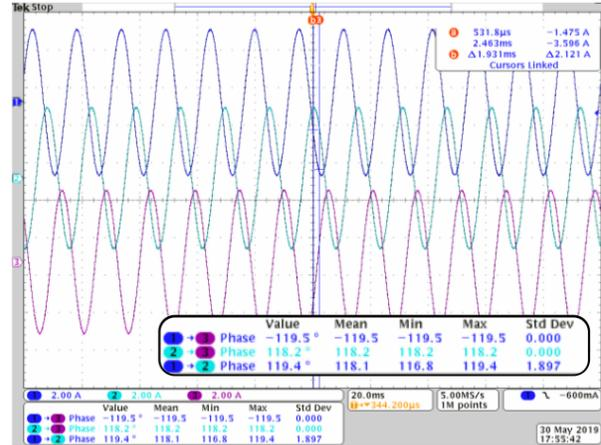
Figure 5.13: Check of phase shift between  $ABC$  winding voltages.
