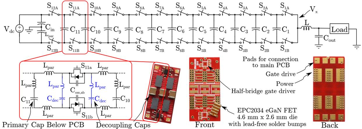
Figure 3.1: Full inverter schematic. Lower left inset highlights the use of small decoupling capacitors immediately adjacent to the GaN FETs to reduce the effective parasitic inductance at the switching nodes. Lower right inset gives closeup of switching cell fabricated on a 0.4 mm PCB with ENIG finish.
