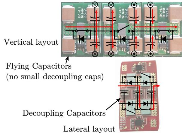
Figure 5.27: Comparison of the vertical and horizontal FCML switch layout. The small decoupling capacitors are replaced by larger flying capacitors in the vertical design.
