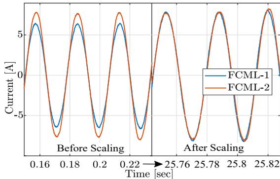
Figure 5.7: Measured FCML AC current before and after modulation depth scaling.
