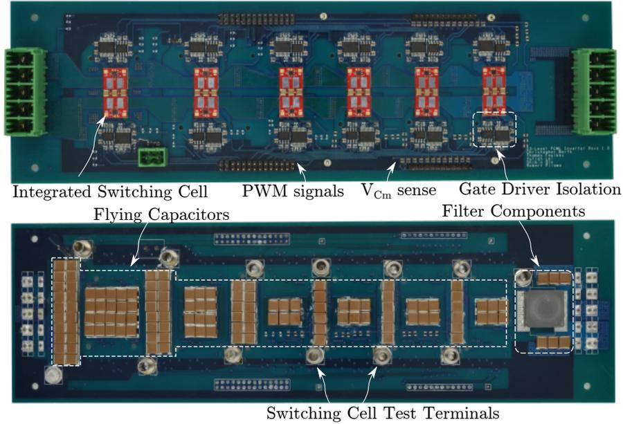
Figure 3.8: Annotated photographs of top and bottom of inverter.
