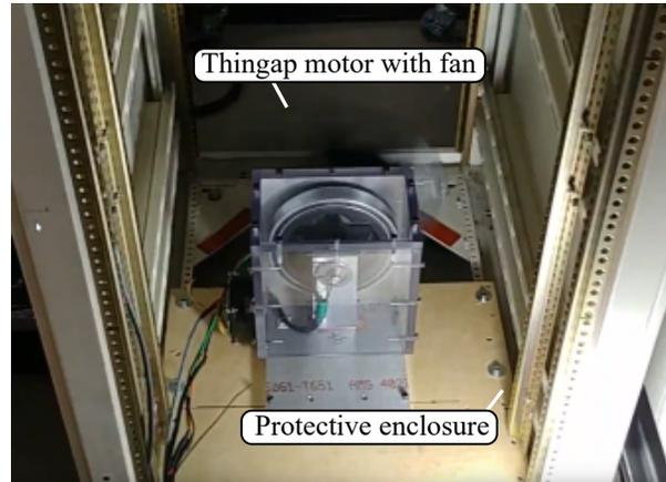
Figure 5.63: ThinGap motor with fan mounted in protective enclosure.
