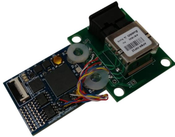
Figure 5.34: Optical transceiver breakout attached to slave controller on Gen 2 ILM. This configuration was used to test the asynchronous serial communication which had been modified for use with optical transceivers.
