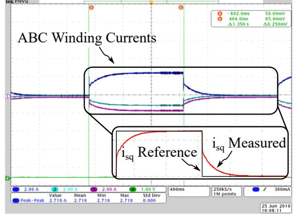
Figure 5.48: Overdamped  $i_{sq}$  step response in  $ABC$  and  $dq$  winding currents with rotor stationary.  $ABC$  winding currents are measured using oscilloscope and  $q$ -axis current read from master controller.
