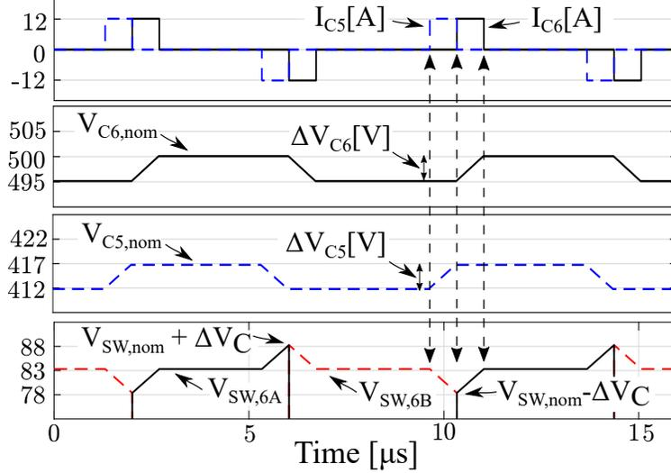
Figure 3.4: PLECS simulation showing charge and discharge of capacitors 5 and 6 in the 13-level inverter at 50% duty ratio. The voltage stress on switches 6A and 6B is increased during the intervals of voltage mismatch between the capacitors as C5 and C6 sequentially charge or discharge.
