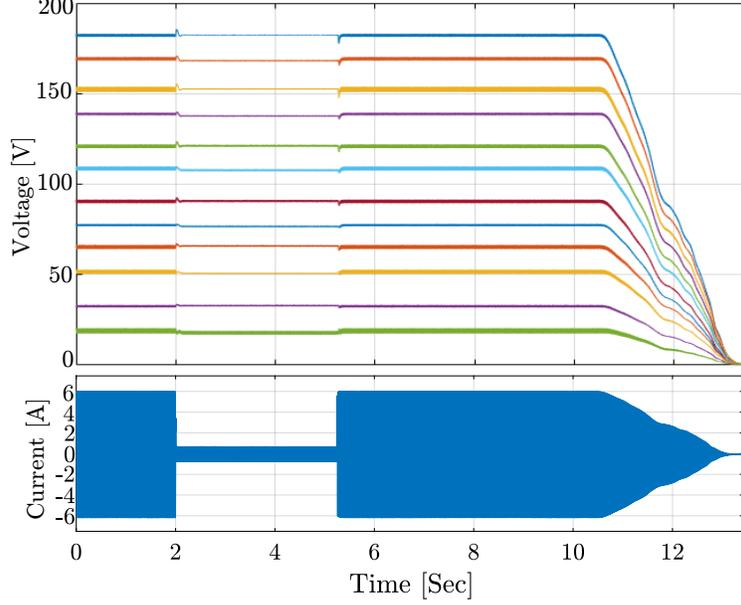
Figure 3.9: Experimental waveforms of capacitor voltage, showing that the 13-level FCML maintains excellent passive capacitor voltage balancing even in the presence of a step load from  $1 A_{pk}$  to  $5.5 A_{pk}$ . Upper plot shows 12 capacitor voltages for the converter operating off of a 200 V bus. Below the capacitor voltages the envelope of the load current can be seen.
