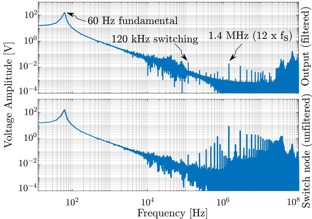
Figure 3.16: FFT of the measured filtered line voltage and the unfiltered switching node voltage.
