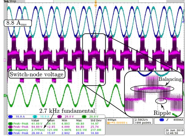
Figure 5.40: Capacitor voltage balancing at 2.7 kHz fundamental with 8.8 A<sub>RMS</sub> load current. Voltage balancing is maintained.
