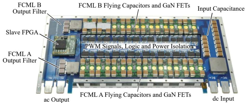
Figure 5.28: Generation 1 of Interleaved Inverter Modules (ILMs) incorporating dual, interleaved, 9-level FCMLs [12].
