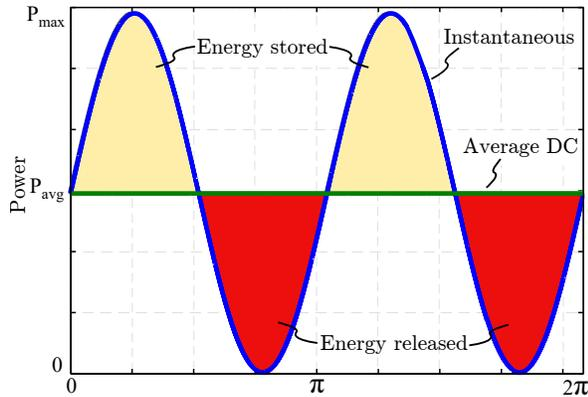
Figure 2.1: Comparison of instantaneous power presented by single-phase AC at twice the line frequency and the average DC power over one power line cycle.
