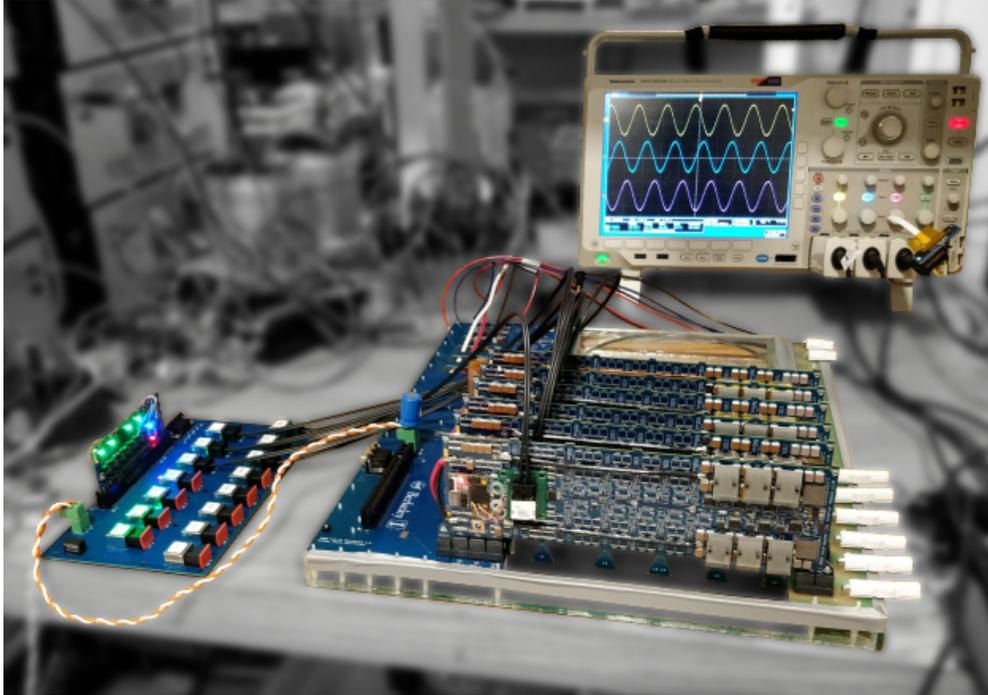
Figure 5.36: Version 2 the modular drive system. Six, 4-level FCMLs combined in a single backplane. Master-slave communication is built into the backplane using RS-485 protocol and the system was adapted to optical communication for final testing.
