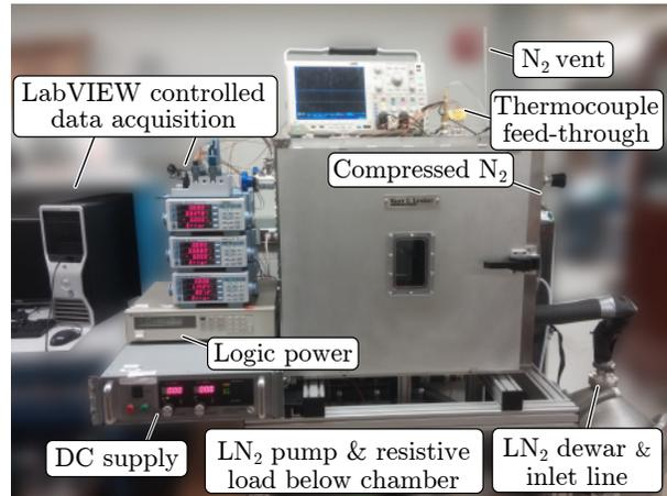
Figure 4.10: Complete cryogenic experimental setup with NI LabVIEW data acquisition.
