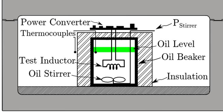
Figure 4.5: Cooler-housed calorimetric measurement system cutaway. Power converter replaced with DC source for calibration.
