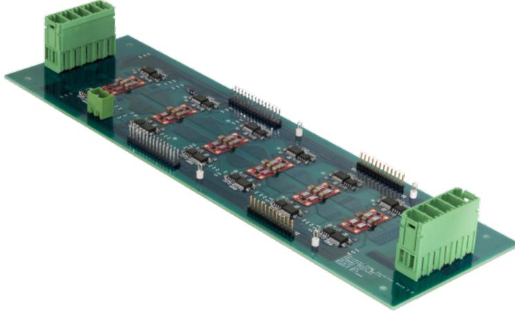
Figure 1.4: 13-level FCML converter used to demonstrate capacitor voltage balancing at high level count.
