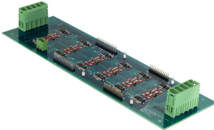
Figure 3.7: Complete 13-level FCML inverter.
