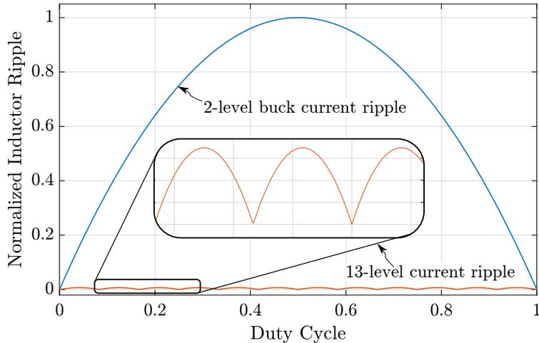
Figure 3.6: Normalized relative inductor current ripple amplitude for two-level and thirteen-level converter with equal DC bus voltage, switching frequency, and inductance.
