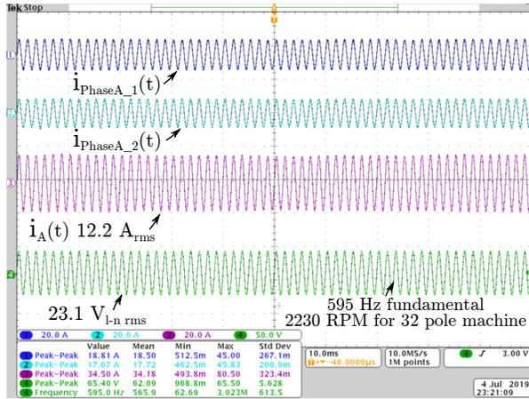
Figure 5.51: Two ILMs driving the ThinGap machine at 2.95 Nm of torque, 2200 RPM.
