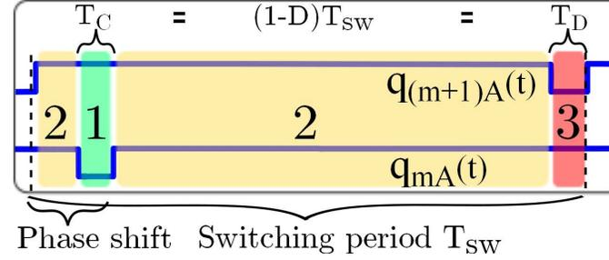
(c) For  $D > 1 - \frac{1}{N-1}$  the charge and discharge is proportional to  $1 - D$ .
