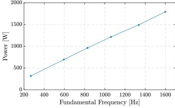
Figure 5.54: Demonstrated motor power vs speed for 4-level modular inverter (2 ILMs per phase) system.
