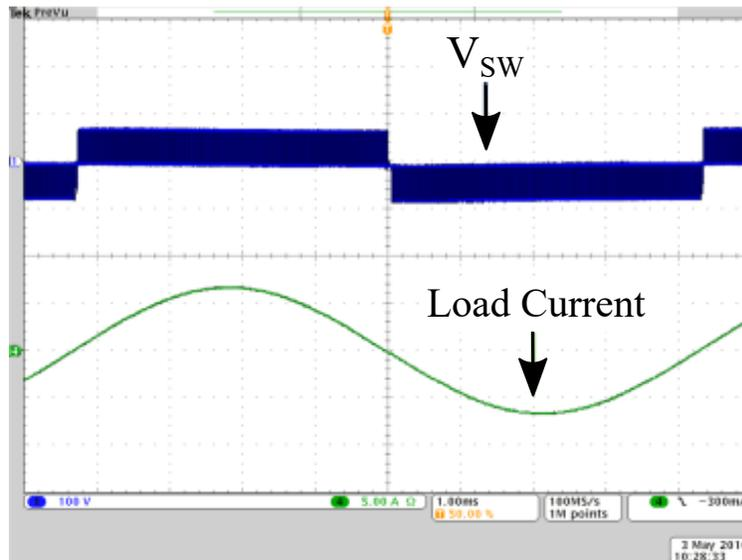
Figure 4.11: Waveforms showing the output current and the switching node voltage ( $V_{sw}$ ) of the 3-level GaN converter.
