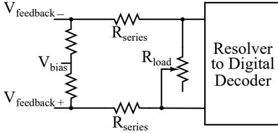
Figure 5.17: Resolver loading circuit used to match feedback amplitude. A separate circuit is used to adjust the amplitude of each resolver signal.
