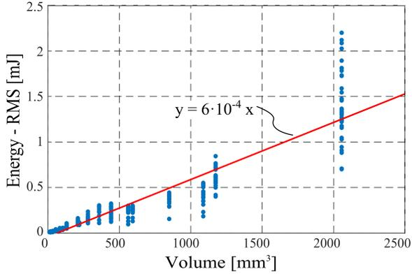
Figure 2.14: RMS energy storage as a function of inductor volume for the IHLP inductor series by Vishay [45].
