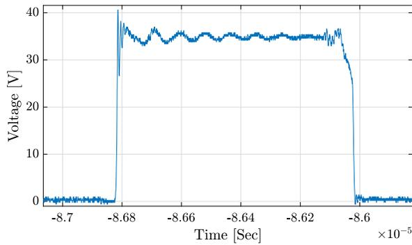
Figure 3.12: Minimal gate-source ringing at switch transition.
