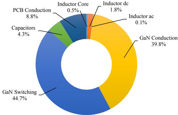
Figure 3.10: Estimated distribution of losses for 13-Level FCML inverter operating at 800 Vdc, 250 Vac, 3 kW.
