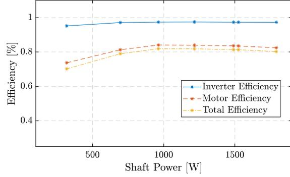
Figure 5.55: Demonstrated efficiency vs power of the combined 4-level modular inverter (2 ILMs per phase) and motor.
