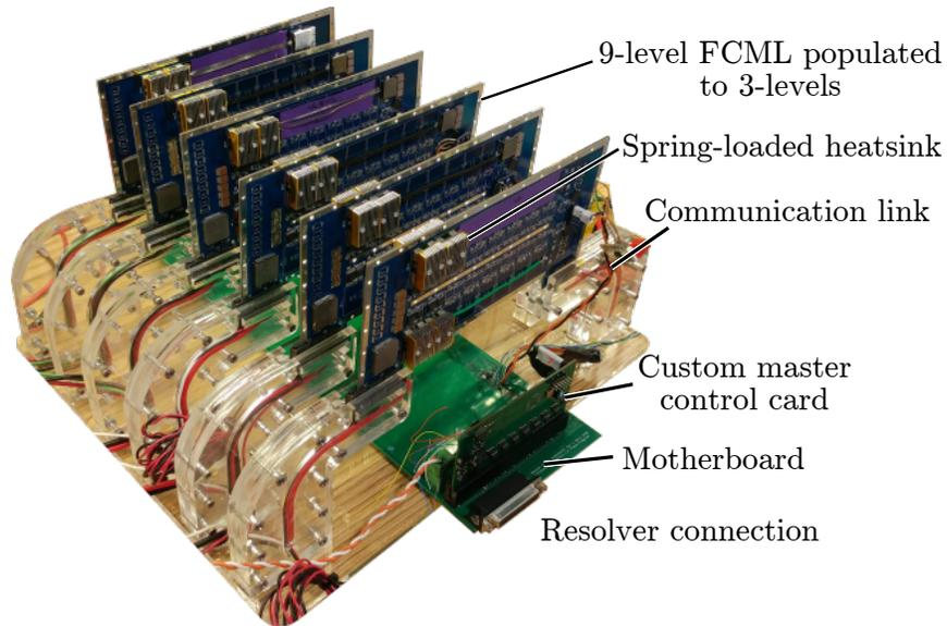
Figure 5.32: Version 1 of FCML-based drive system. Six, 3-level FCMLs assembled into a 3-phase inverter using an acrylic frame.
