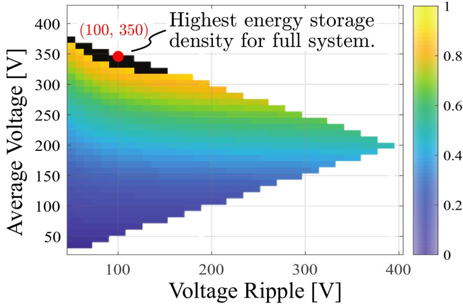
Figure 2.17: Normalized relative energy density over ripple and average voltage for a full system including bias-independent capacitors, inductor and heatsink. Black region indicates top 10% of density. It can be seen that the maximum energy density occurs at high average voltage.
