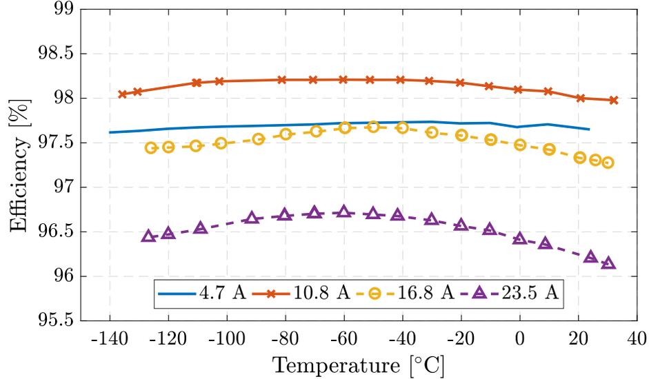
Figure 4.13: Measured efficiency versus temperature for four different load levels. At light load the converter losses are dominated by switching and therefore there is minimal change in efficiency with temperature.
