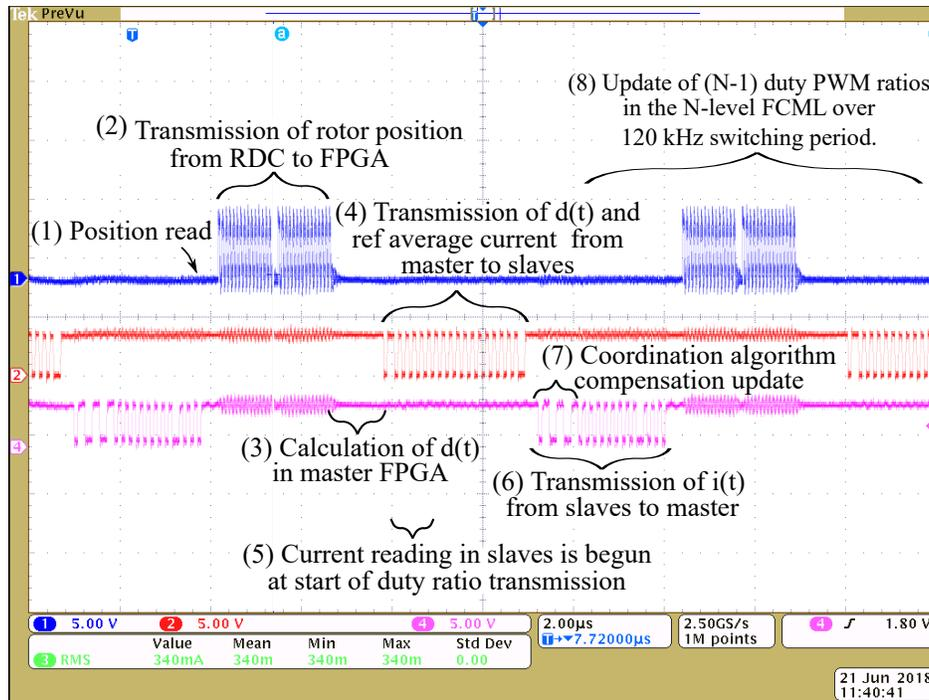
Figure 5.23: Duty ratio update sequence shown in the context of communication between the resolver decoder, master controller, and slave.
