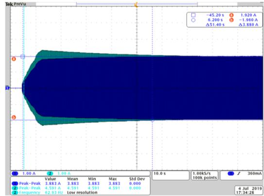
Figure 5.44: Duty ratio compensation used to evenly distribute load current.
