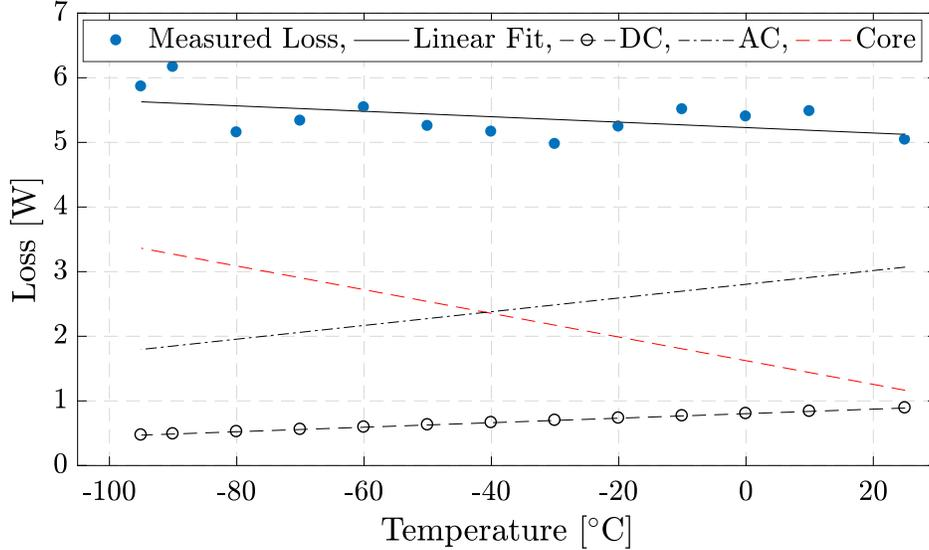
Figure 4.6: Electrically measured losses for two parallel inductors in dc-dc test.  $V_{in} = 100$  V,  $D = 0.75$ ,  $I_{load} = 7.4$  A,  $I_L = 8.3$  A<sub>RMS</sub>,  $F_{sw} = 70$  kHz,  $F_{effective} = 140$  kHz. It is observed that the overall losses remain relatively stable indicating that core losses increase to account for the difference between the measured loss and the known decrease in conduction and AC losses based on the temperature coefficient of copper.
