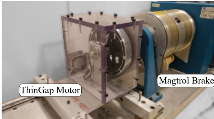
Figure 5.46: Magtrol hysteresis dynamometer with mounted ThinGap motor.
