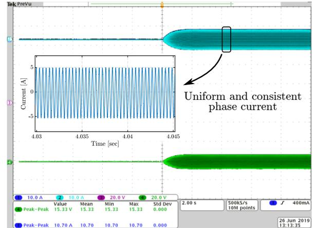
Figure 5.42: Current on phase A during  $i_{sq}$  ramp. Data captured concurrently with Fig. 5.41.
