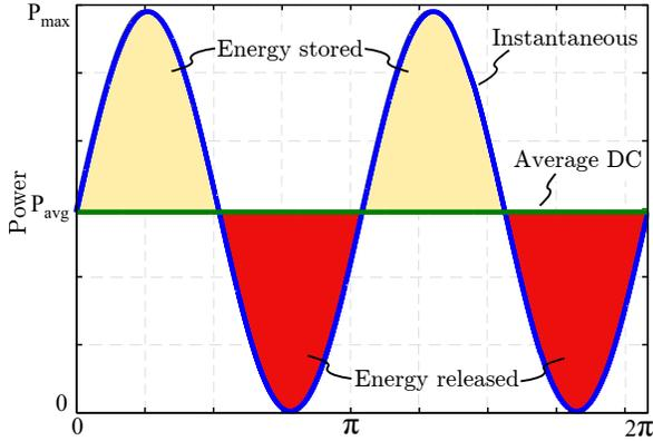
Figure 1.2: Instantaneous power mismatch between DC and single-phase AC.
