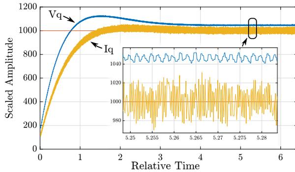
Figure 5.41: Ramp of q-axis voltage and current into a resistive load for demonstration. Time stamp from master controller is approximate.
