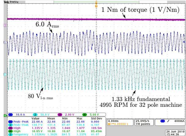
Figure 5.50: Waveforms from driving the ThinGap motor at 5 kRPM.
