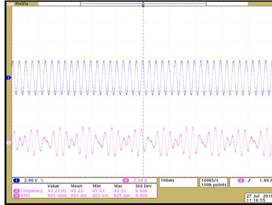
Figure 5.15: Motor current even sinusoidal voltage and oscillation in current amplitude resulting from oscillating phase shift.
