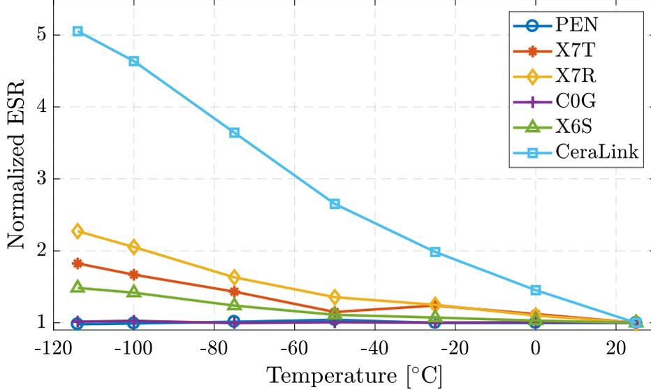
Figure 4.4: Measured large signal ESR over temperature normalized to ambient value for several different capacitor dielectrics. Measurements are taken using the large signal test outlined in [6].
