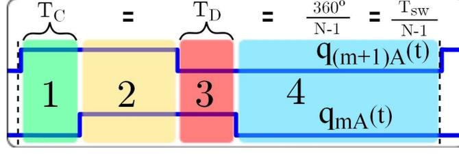
(a) Within the range  $\frac{1}{N-1} < D < 1 - \frac{1}{N-1}$ , the charge and discharge interval is set by the phase shift.
