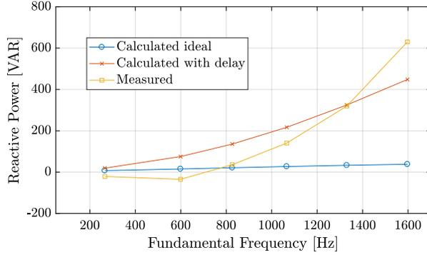
Figure 5.58: Comparison of reactive power drawn by ThinGap motor in lab measurements against reactive power based on motor parameters with in-phase and delayed excitation.
