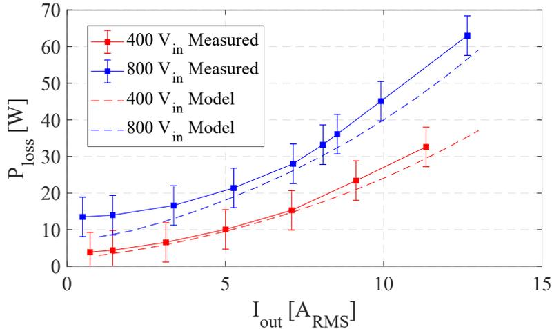
Figure 3.14: Total measured plotted along with model-based estimates of loss.
