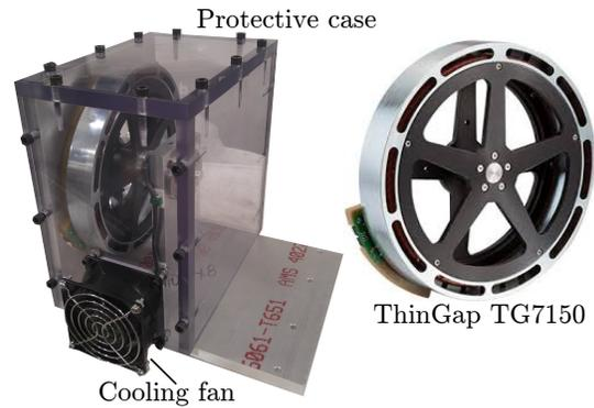
Figure 5.2: ThinGap 32-pole test machine mounted in enclosure [130].
