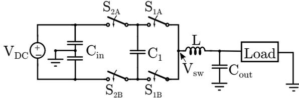
Figure 4.1: Schematic drawing of the 3-level GaN FCML inverter.
