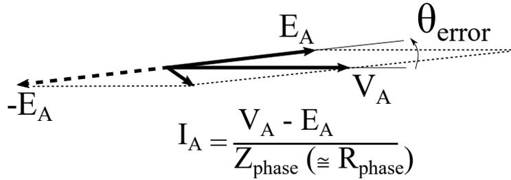
Figure 5.56: Delay in inverter applied voltage ( $V_A$ ) results in increased lagging line current and inductive reactive power flow.
