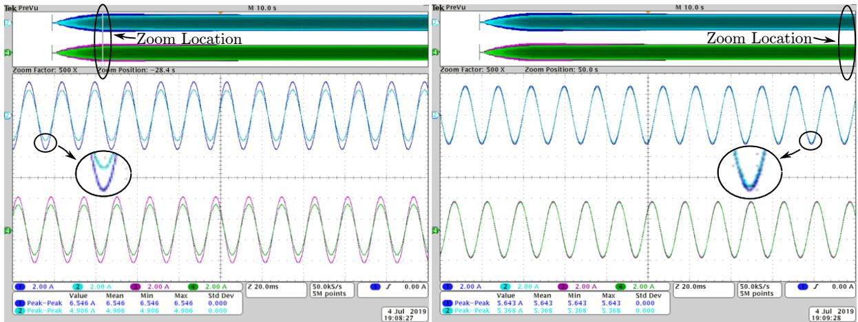
Figure 5.45: Converging current amplitude for 2 phases in a 3-phase system. Slow proportional control is used to compensate for a 30% load mismatch in roughly 90 sec.
