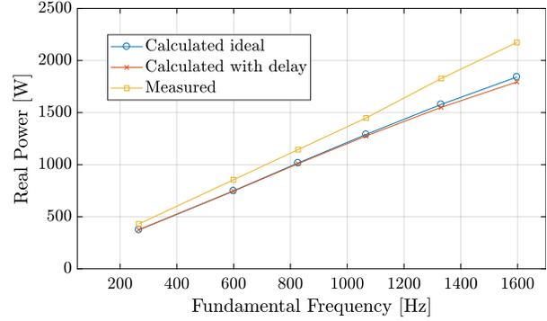
Figure 5.59: Comparison of real power drawn by ThinGap motor in lab measurements against real power based on motor parameters with in-phase and delayed excitation.
