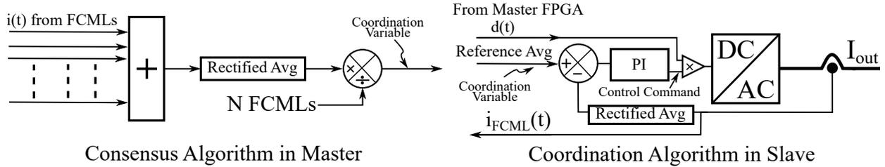
Figure 5.6: Consensus and coordination algorithm operating in master and slave.
