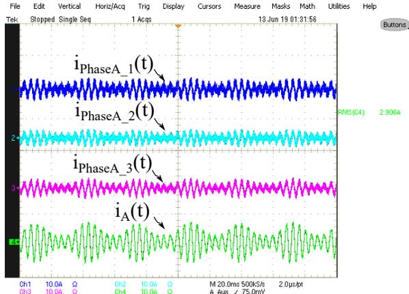
Figure 5.62: Combined phase A current from three ILMs operating in parallel. Ripples in current amplitude are the result of driving the ThinGap motor at light load.
