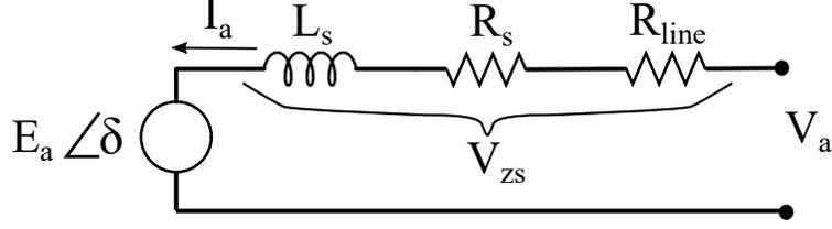
Figure 5.57: Single-phase equivalent circuit for PM machine.
