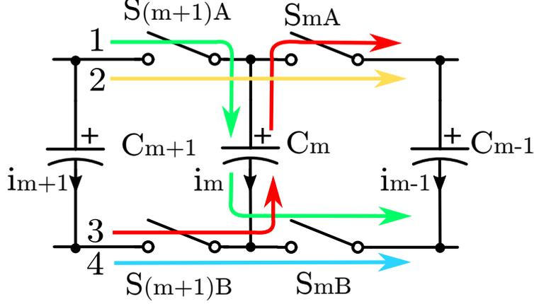
Figure 3.3: Subcircuit depicting the current flow in different switch configurations. The charge/discharge of capacitor  $C_m$  is entirely dictated by the positions of switch sets  $S_m$  and  $S_{m+1}$ . Switches A and B are always complementary, in order to maintain a voltage difference between capacitors.
