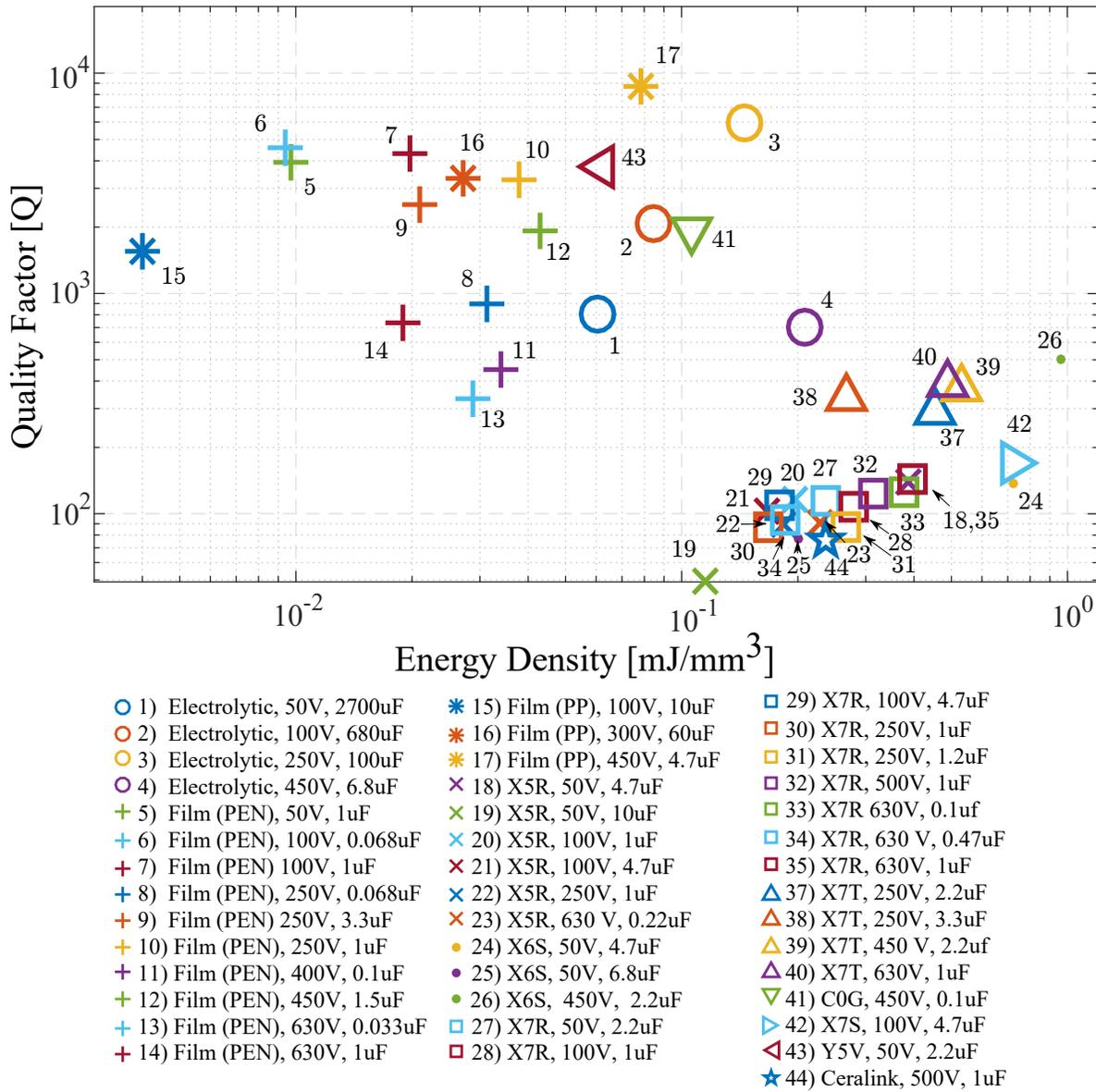
Figure 2.10: Capacitor Q vs. energy storage density.
