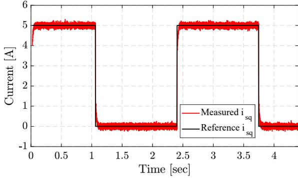
Figure 5.47: Critically damped  $i_{sq}$  step response during tuning of the  $i_{sq}$  and  $i_{sd}$  controllers. Both reference and measured values read from the master controller.
