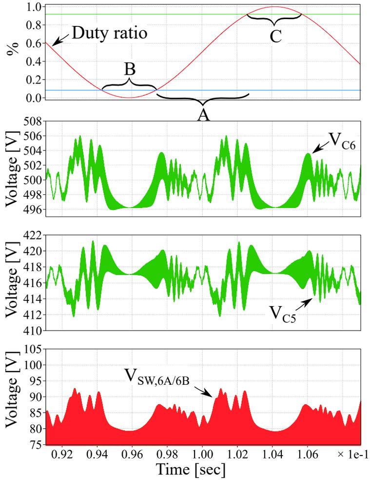
Figure 3.5: PLECS simulation showing switch blocking voltage for the 13-level converter operating at 350 V<sub>RMS</sub>, 8.6 A<sub>RMS</sub>. It can be seen that switch blocking voltage is maintained in a safe region and that the interval  $\frac{1}{N-1} < D < 1 - \frac{1}{N-1}$  (Region A) is the region of highest capacitor voltage ripple as outlined in Fig. 3.2.
