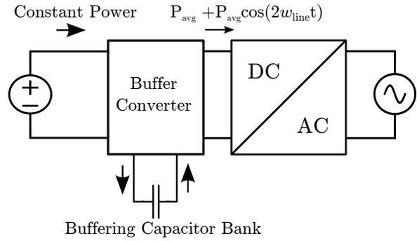
Figure 1.3: Energy buffering circuit of single-phase inverter.
