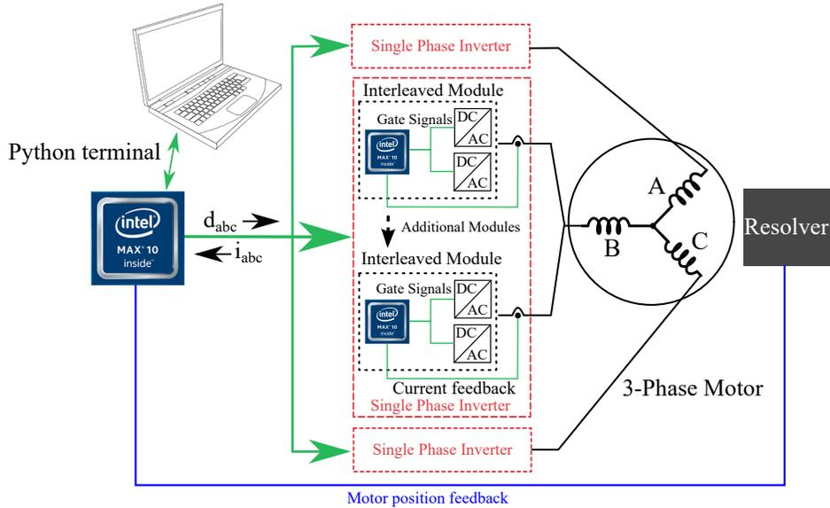
Figure 5.4: High-level hierarchical control structure for FCML-based motor drive system. Master controller sends reference duty ratio to slave controllers based on measured motor position and current feed-back from slaves.
