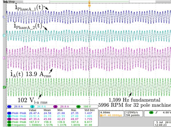
Figure 5.53: Two ILMs jointly driving the ThinGap machine at 2.85 Nm of torque, 5996 RPM. Some oscillations are present in the phase current.
