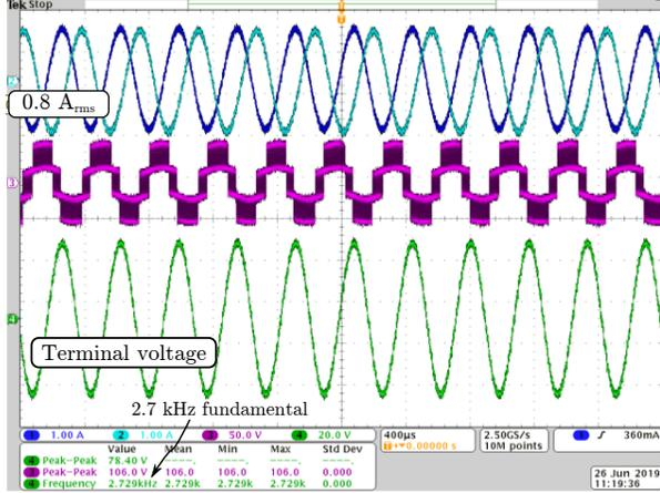
Figure 5.39: Capacitor voltage balancing at 2.7 kHz fundamental with 0.8 A<sub>RMS</sub> load current. High fundamental frequency has negligible impact on voltage balancing.
