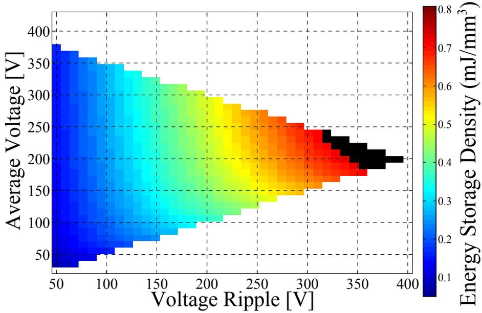
Figure 2.12: Energy buffering density for the 2.2  $\mu\text{F}$ , 450V, X6S capacitor #26. Black region indicates top 10% of energy density. In the bias-dependent buffer configuration note that the maximum energy density still occurs at high voltage ripple, but the average voltage is shifted slightly down. Exploring the implications of this shift is the focus of this section.
