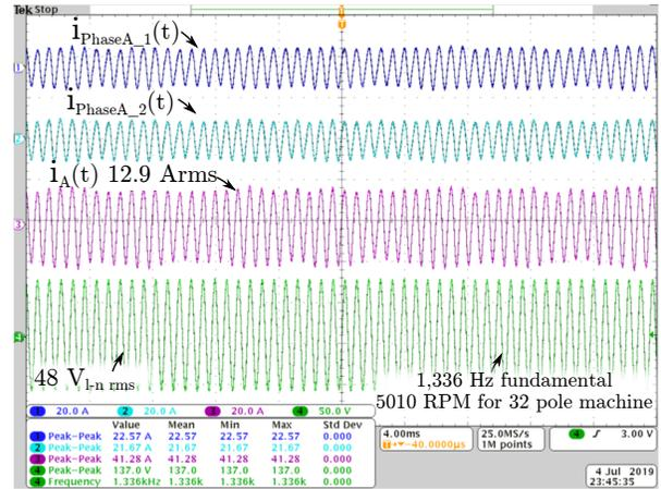
Figure 5.52: Two ILMs driving the ThinGap machine at 2.85 Nm of torque, 5010 RPM.
