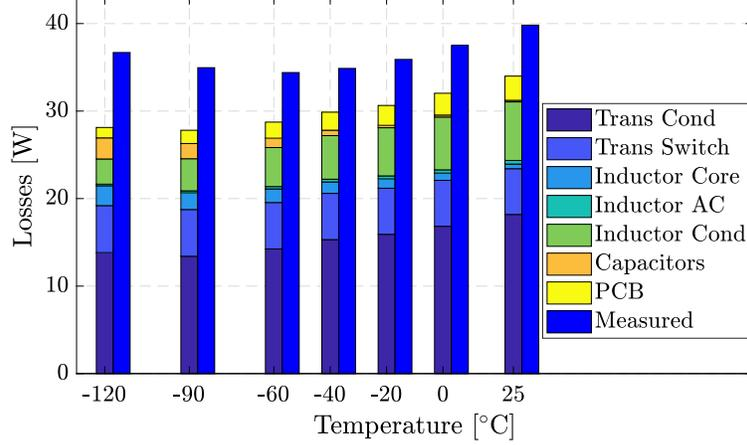
Figure 4.14: Measured power losses and estimated losses versus temperature at (23.5 A<sub>RMS</sub> output). Although the losses are under estimated by the model, the trend is in agreement.
