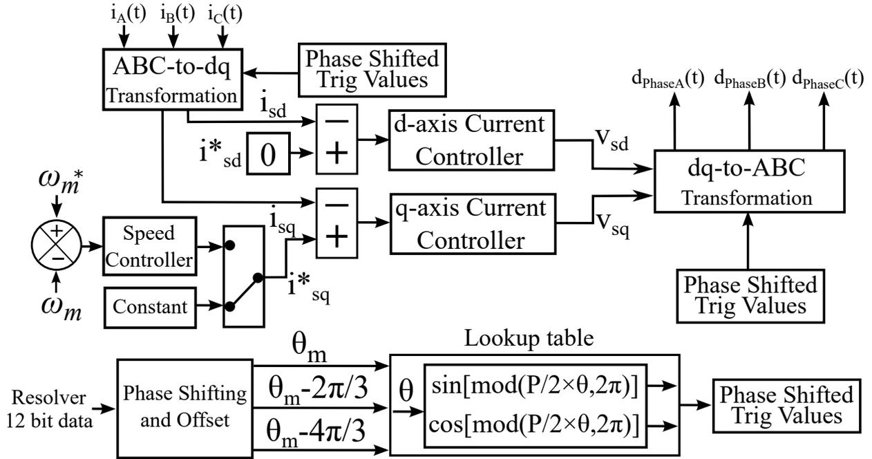
Figure 5.21: Vector control module used to generate phase voltages.
