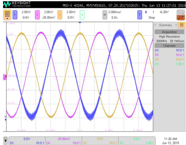
Figure 5.61: Three-phase voltage from set of 10-level ILMs operating in parallel.
