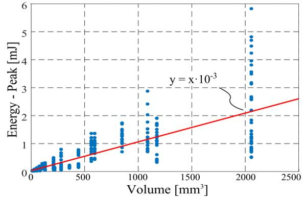
Figure 2.15: Peak energy storage as a function of inductor volume for the IHLP inductor series by Vishay [45].
