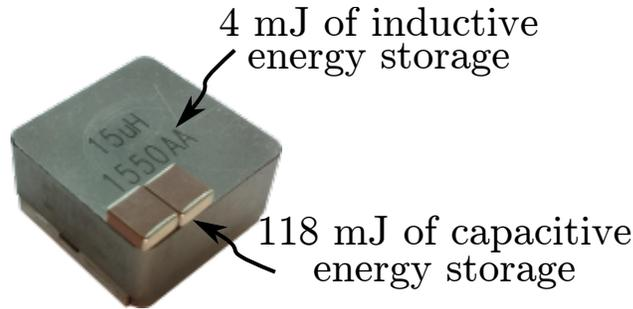
Figure 1.1: The energy storage density of capacitors far exceeds that of inductors in most power electronics applications.
