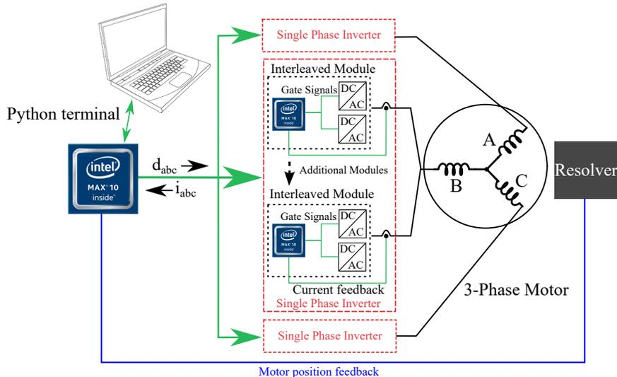
Figure 1.6: Structure of FCML-based motor drive system.
