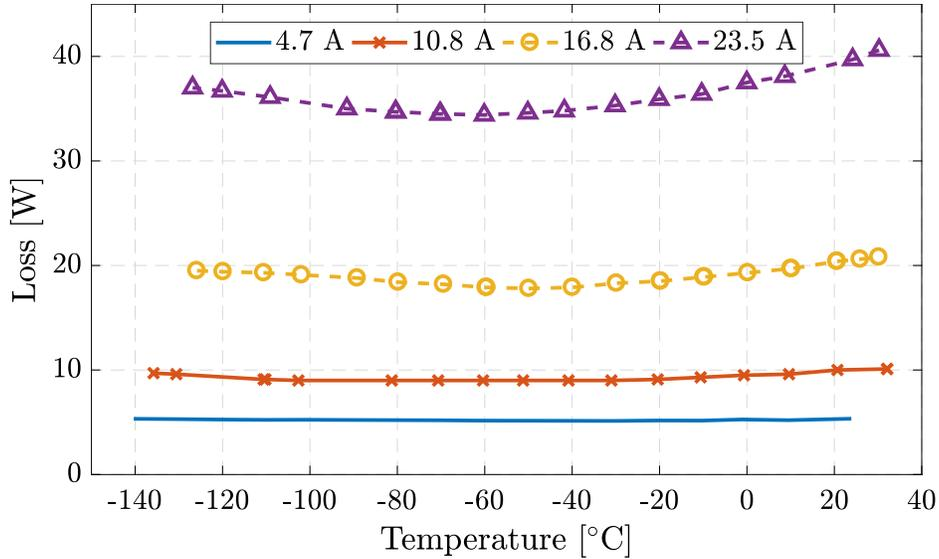
Figure 4.12: Converter losses at four different loads. At higher load conduction losses dominate and there is a measurable decrease in losses down to  $-60\text{ }^{\circ}\text{C}$ .
