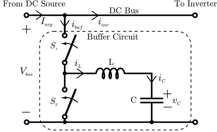
Figure 2.13: Bi-directional buffer converter schematic.
