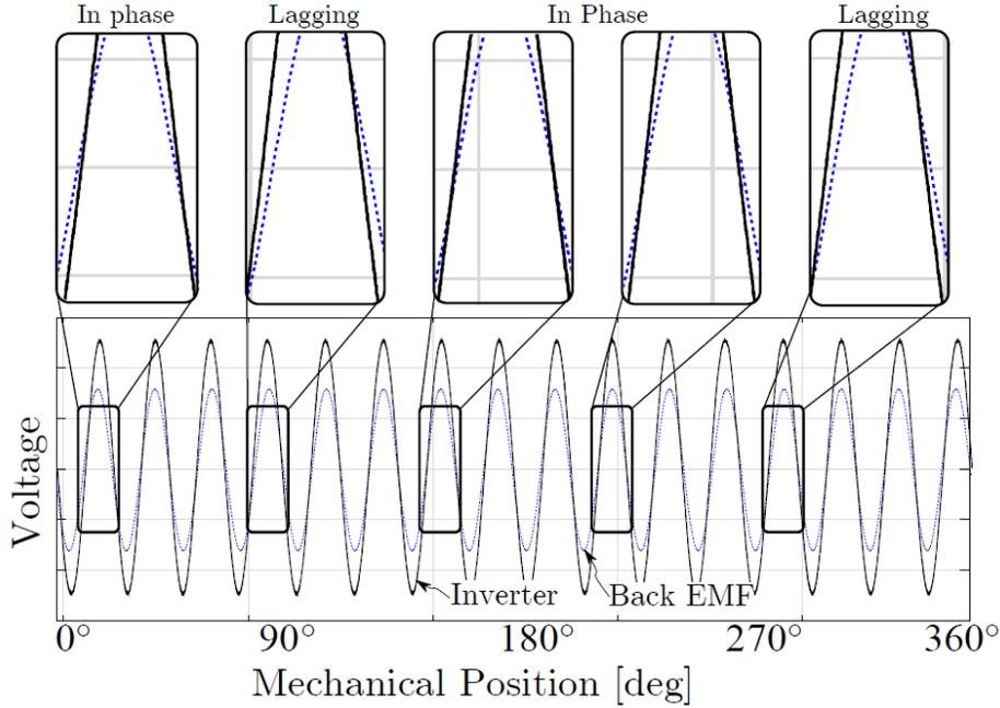
Figure 5.16: Single-phase comparison of inverter voltage and open winding motor back-EMF. Inverter applied voltage lags motor back-EMF twice per mechanical rotation.
