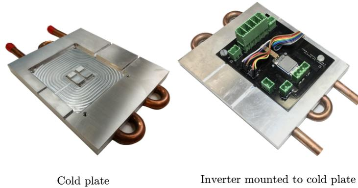
Figure 1.5: Three-level FCML inverter with cold plate for low temperature testing.
