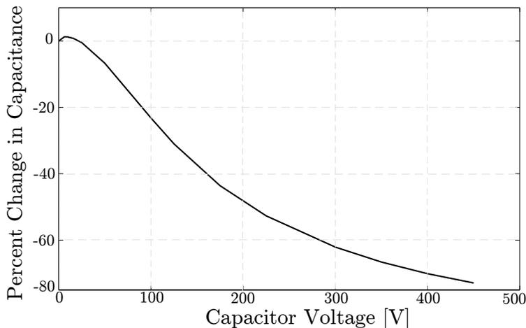
Figure 2.3: Plot of capacitance change vs. bias voltage for TDK CKG57NX7R2J474M500JH capacitor [39].
