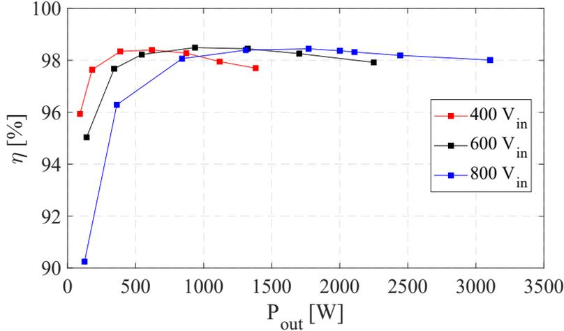
Figure 3.13: Inverter efficiency over load for dc bus voltages of 400 V, 600 V, and 800 V with a constant modulation depth.
