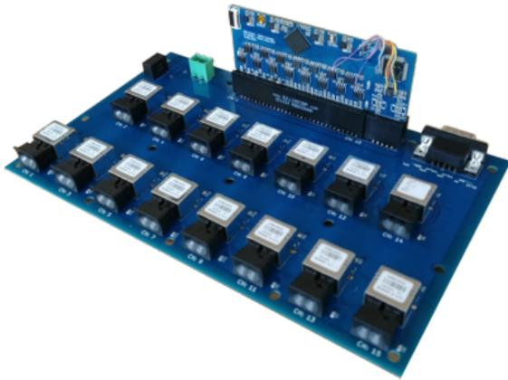
Figure 5.33: Optical adapter board built facilitate communication between master and slave controllers over POF.
