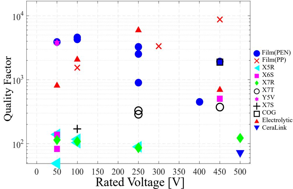
Figure 2.8: Measured capacitor quality factor showing that film capacitors rank among the highest in quality factor.
