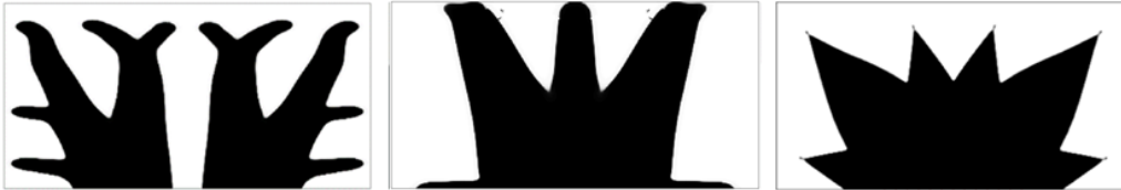
Figure 5.9: SIMP topology optimization solutions for thermal compliance objective. Pure conduction (left), conduction with uniform convection (center), conduction with boundary-dependent convection (right).
