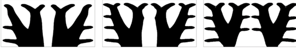
Figure 5.10: Topology optimization solutions for various objective functions. Thermal compliance (left), maximum temperature (center), temperature variance (right).
