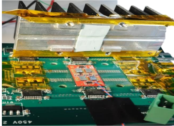
Figure 6.1 Multilevel dc-ac converter enclosed with a heat sink. The heat sink is made of Aluminum. A thermal gap pad (Gap Pad 5000S35) is placed on top of the active components between the inverter and the base of the heat sink.
