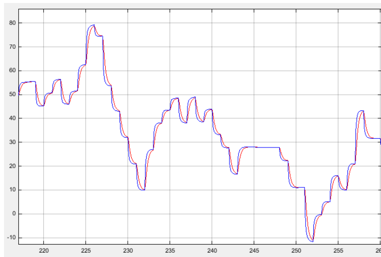
Figure 3.11: I/O of Torque Lag Block - Blue: Input Red: Output
