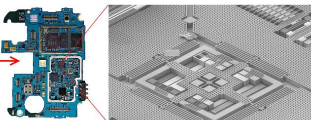
Inside your phone is a chip with a sensor the width of a human hair (~80 microns) that measures how your phone accelerates
