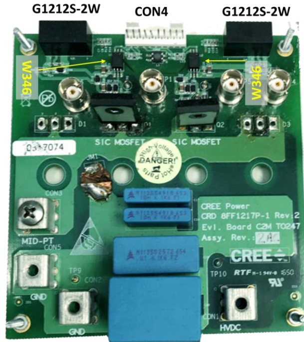
Fig. 6-1. KIT8020CRD8FF1217P half-bridge evaluation board [37].
