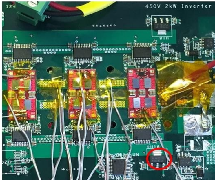
Figure 3.13: Top view of the experimental setup with a faulty component indicated using a red circle located at the right bottom.
