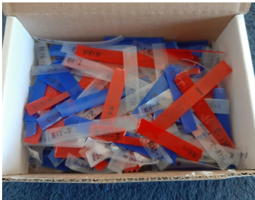
Figure F.4: Film sample set pre- and post-testing. Includes some nylon testing samples that were not used in the final study.
