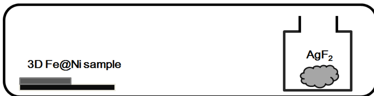
Figure 2.12 Illustration of the fluorination process. The reactor is sealed and under vacuum.
