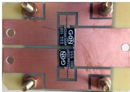
c) Fabricated EMI filter integrated wire-bondless GaN module
