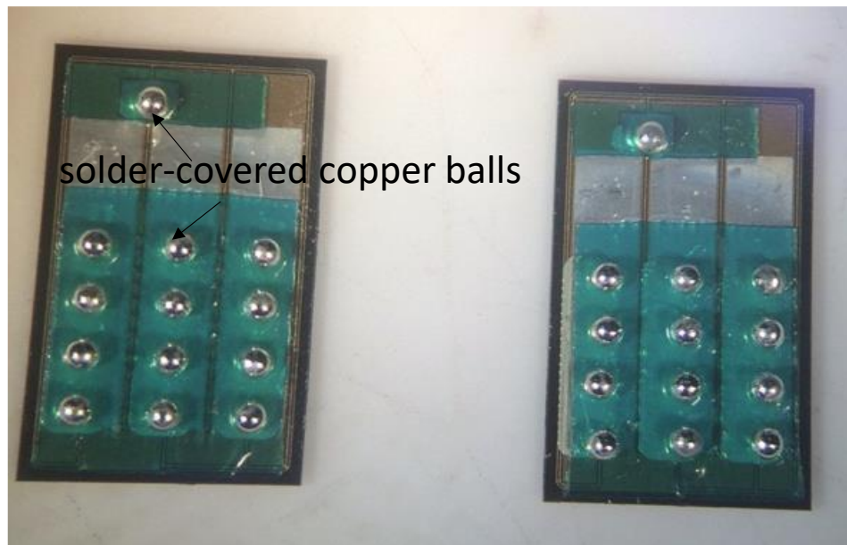
Fig. 3. 7 MOSFET bare dies with copper balls attached on.
