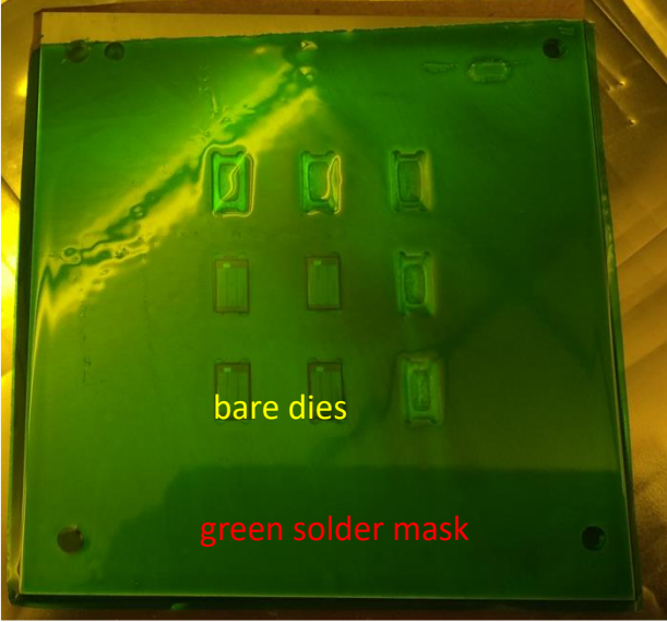
Fig. 3. 5 MOSFET bare dies covered with dry film solder mask.
