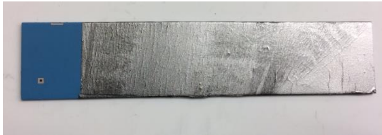
Fig. 5. 6 Fabricated LTCC interposer sample with PGS attached on surfaces.
