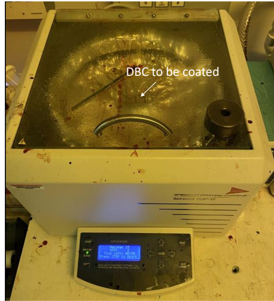
Fig.6. 25 PI coating on die attached DBC substrate using a spin coater.
