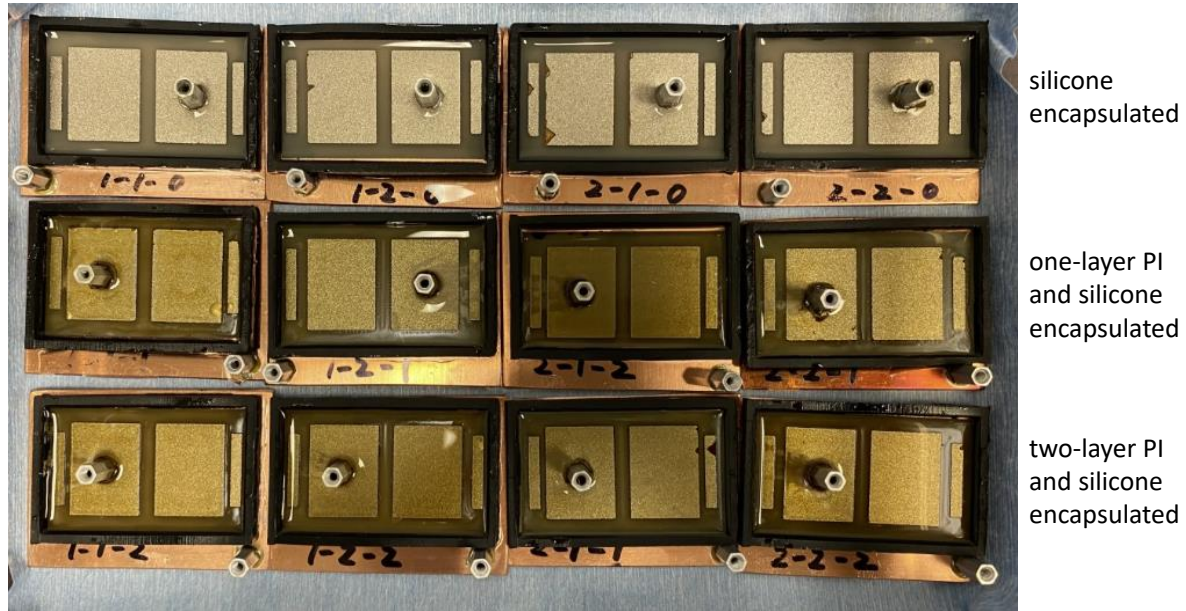
Fig.6. 33 Samples with different encapsulant for high voltage breakdown test.
