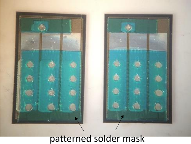
Fig. 3. 5 MOSFET bare dies covered with dry film solder mask.
