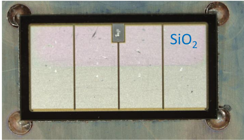
Fig.6. 21 3.3-kV MOSFET bare die with SiO 2 layer deposited.
