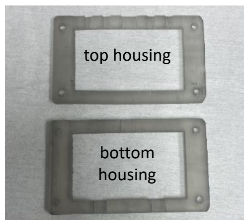
Fig.6. 26 3-D printed high temperature housing.
