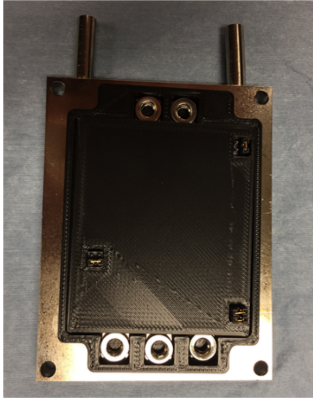
Fig. 5.18: Picture of fabrication process. Step XII, lid placement
