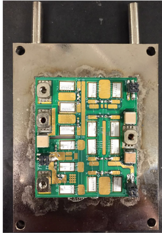
Fig. 5.16: Picture of fabrication process. step VII (left), wire bonding. IX (right): terminal, screw, gate resistor, and multi-layer ceramic capacitor placement.
