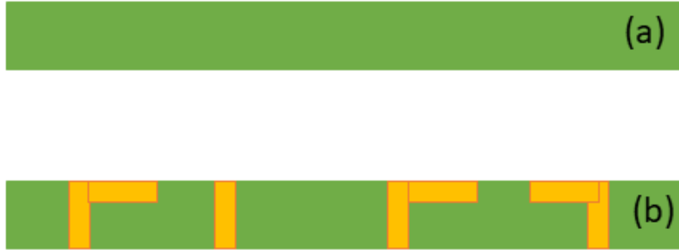
Figure 4-1: (a) Modeled shape of PCB (b) Actual shape of PCB highlighting internal components
