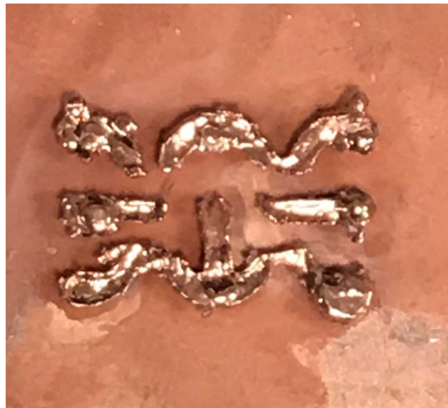
Figure 3-8: (a) Image of fabricated compliant interconnects within the mold (b) Image of compliant interconnects after mold removal
