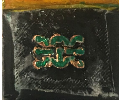
Figure 3-12: Exposed dry film on a fabricated sample
