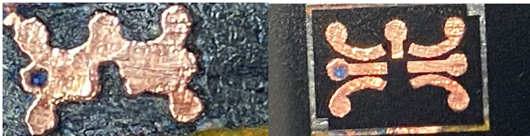
Figure 3-13: Optical images of interconnects (a) before polishing (b) after polishing
