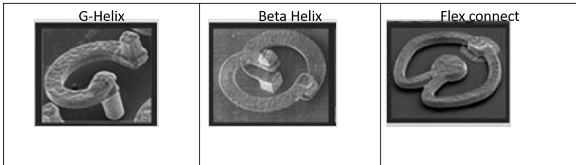
Figure 2-6: SEM images of different compliant interconnect geometries G-Helix [54], Beta Helix [55], Flex connect [56]
