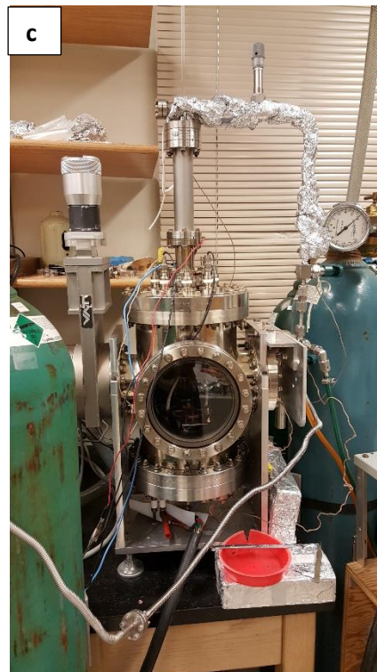
Figure 25: (a) Device structure used for the nanosoldering experiment (side view). (b) Top view of figure 25 (a). (c) Turbo chamber used for the nanosoldering experiment.
