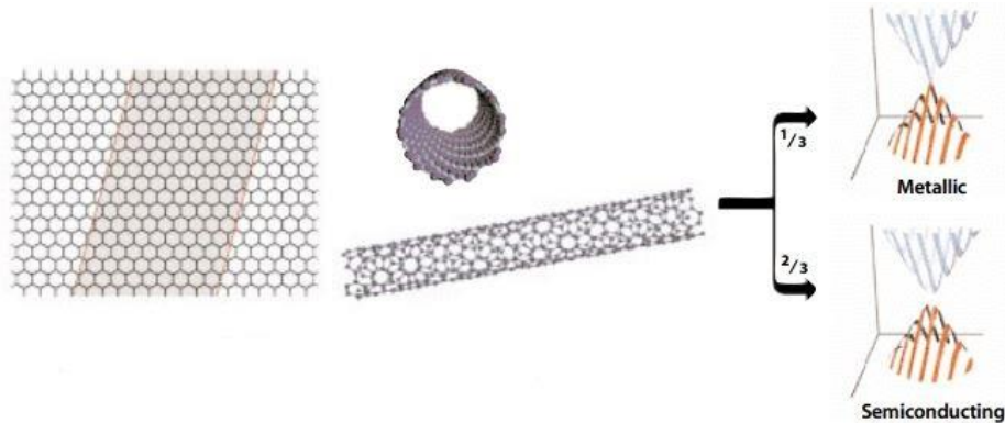
Figure 3: A schematic illustration of a graphene sheet being rolled up into a CNT. Depending on how the sheet is rolled up, the resulting CNT can be either semiconducting or metallic. [7]
