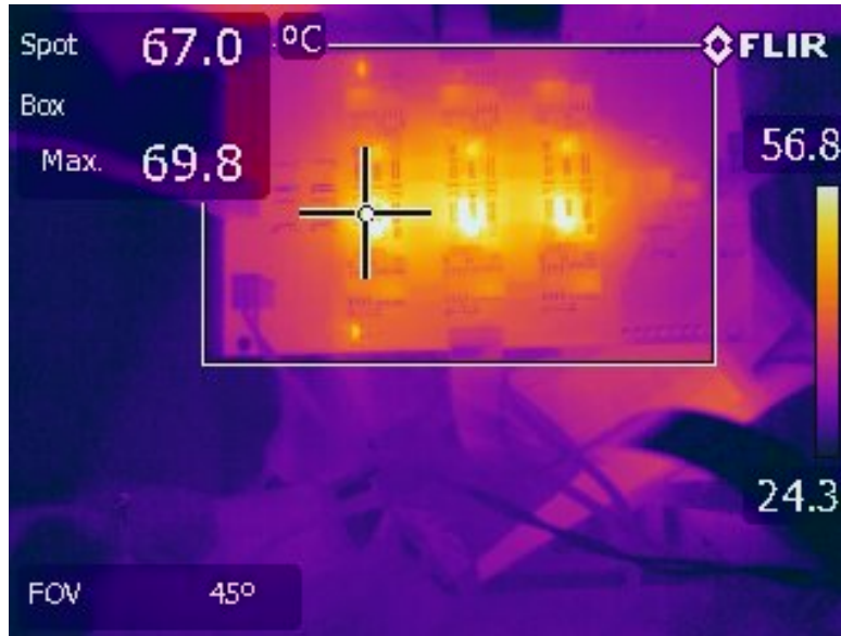
Figure 4.9: Heat distribution in converter: hard switching. P_{out} = 150\text{ W} .
