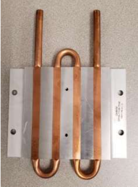
Figure 31 A Picture of the Cold Plate (Ohmite CP4A-114B-108E) Used in This Work
