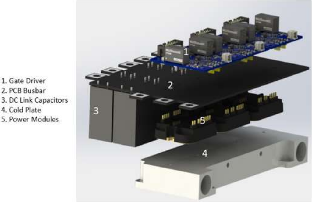
Figure 54 Final Inverter System Design (Exploded)
